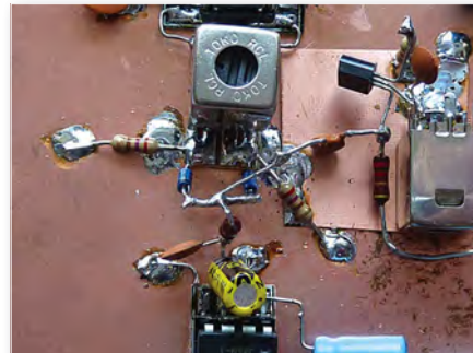
There is no amplification at the i.f. from the first mixer, just a tuned matching transformer. This and the b.f.o. feed a double diode second mixer and the audio output goes straight to the input of the LM386.
