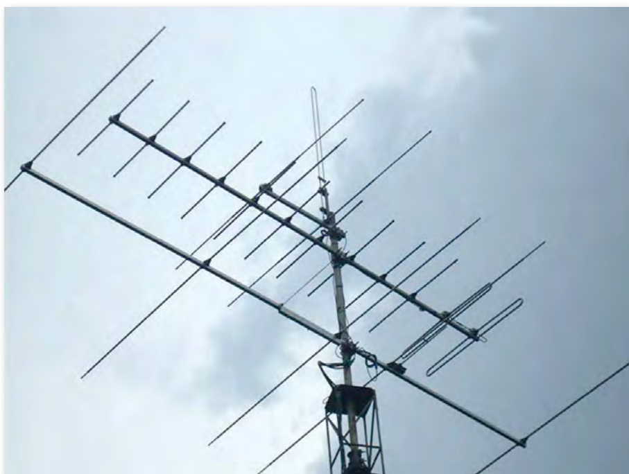
Fig. 3: The two-element HB9CV antenna built and installed by Owen Wheeler, G0NCE, can be seen on his mast above his 50MHz and 144MHz yagis.
