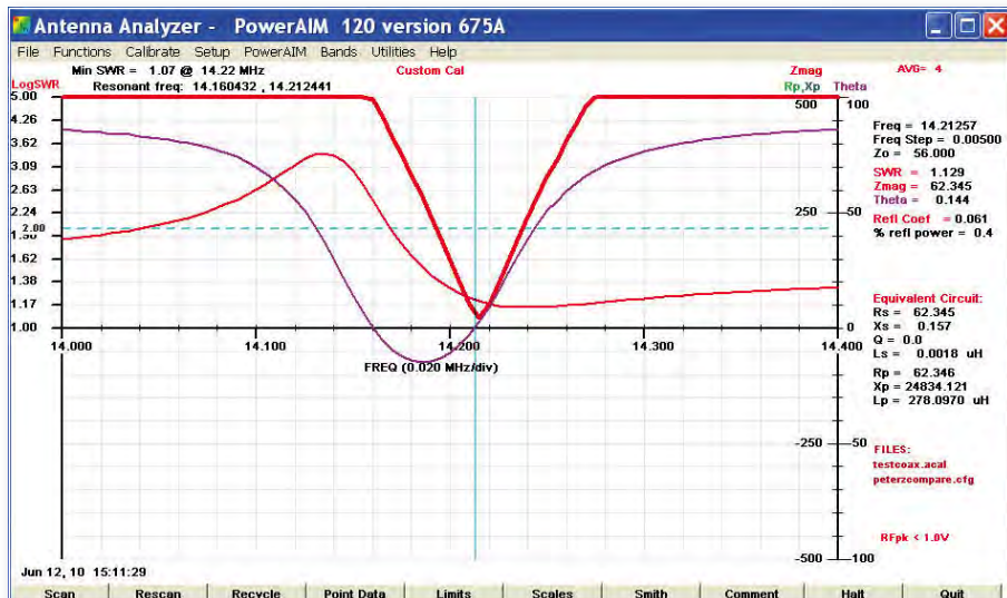
Fig 4: Measurements of s.w.r., Z magnitude and Theta of the finished loop using the AIM 4710.
