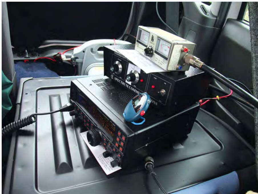
The setup for GOBWC/P was a 'com IC-7000 transceiver with a Spectrum transverter, feeding a home-brew 5-element yagi antenna, with 'Armstrong rotator'.
