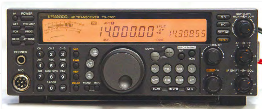
Fig. 2: The Kenwood TS-570D is a typical modern h.f. transceiver with a built-in automatic a.t.u. Output power can be adjusted between five and 100W, making it suitable for those with a Foundation Licence intending to upgrade to an Intermediate and Advanced Licence. It needs an external power supply unit (p.s.u.) for mains operation.
