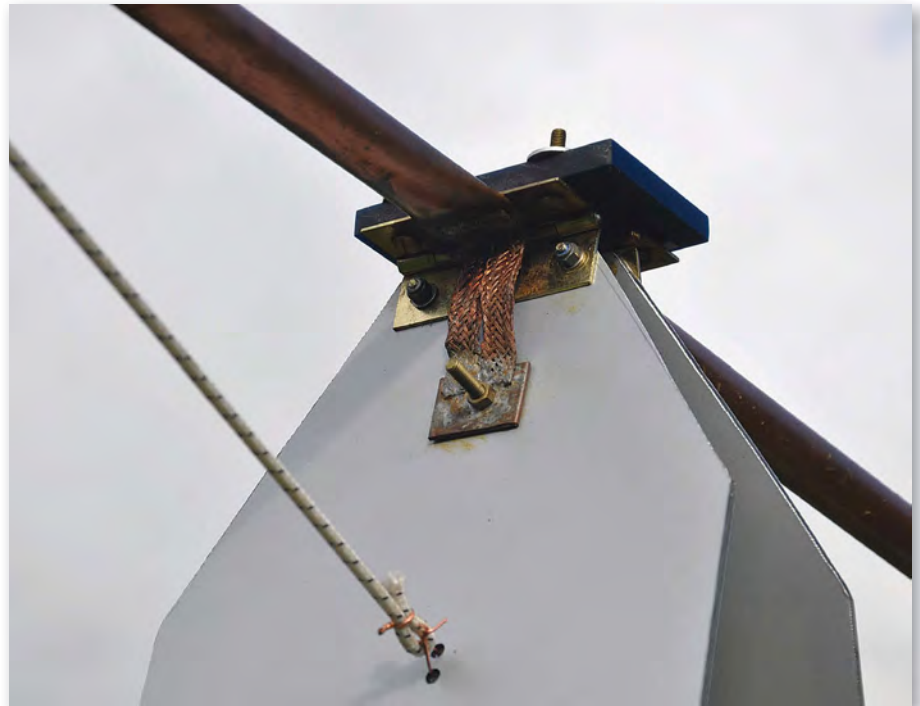
Fig 3: Detail of the capacitor with the coaxial cable braid to provide an r.f. bypass of the hinges.
