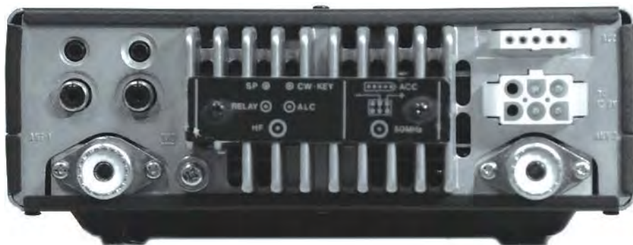
Fig. 4: The rear panel of an Alinco DX-70 showing the separate h.f. and 50MHz antenna and other sockets.
