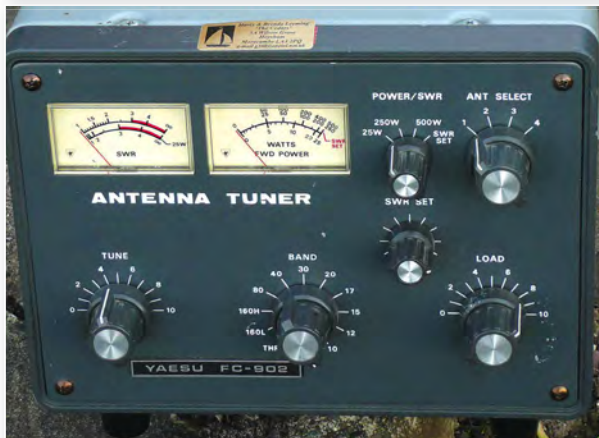
The front panel of what Harry reckons is the peak of antenna matching units - the Yaesu FC-902.
