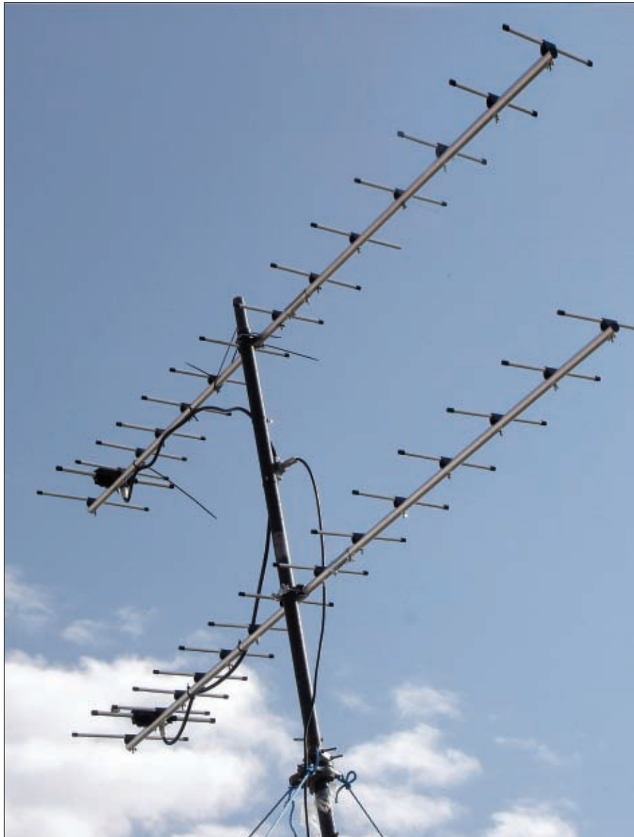
This imposing stacked pair of 430MHz antenna, used for mountain-top portable operations close to the Flabouri shelter in Greece. This was sent in by Panos Dadis SV1GRN of the Athens QRP group.
