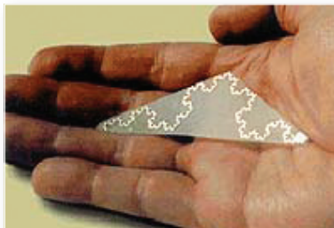
Fractal antenna can be used for multi-band operation on h.f., v.h.f. and u.h.f. as well as higher frequencies.
