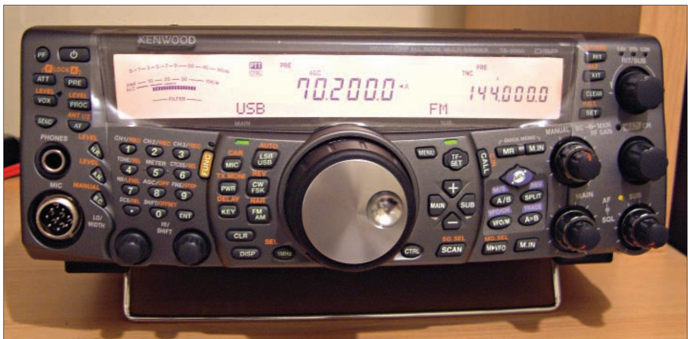
Fig. 1: Kenwood's TS-2000 is a modern compact transceiver covering h.f., v.h.f., and u.h.f. bands with a built-in a.t.u., which can save a lot of space in comparison with separate equipment.
