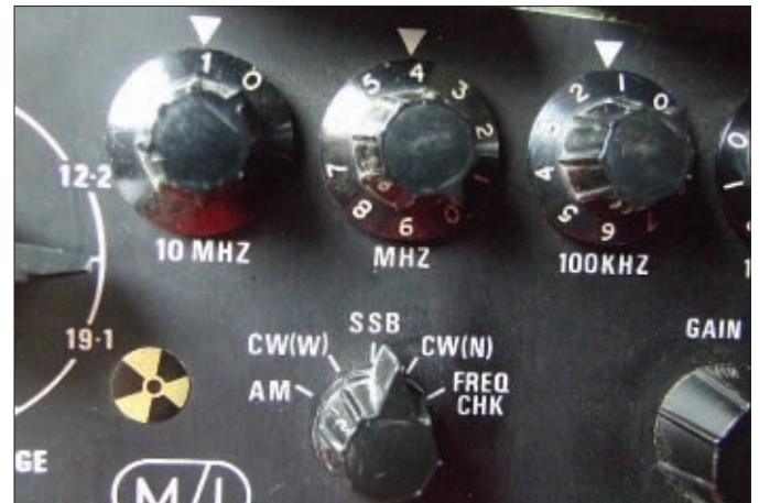
Fig. 4: Showing the mode selections available on the PRC-320.
