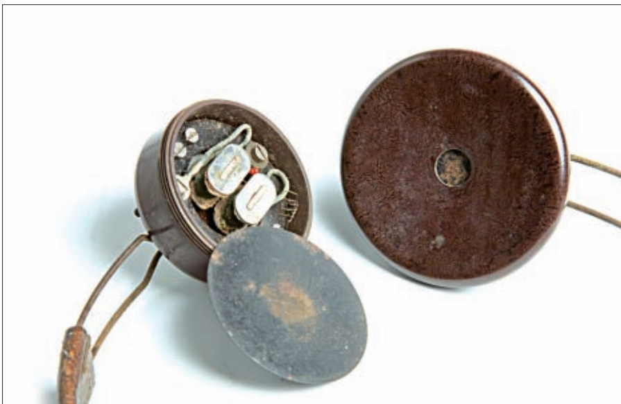
Fig. 1: A photograph of the workings of the older high impedance headphones. The flat plate diaphragm is attracted to the 'pole-pieces' of the electromagnet, which also requires some permanent magnetism to give a reasonable quality audio as explained in the text.
