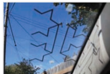
Fractal antenna can be used for multi-band operation on h.f., v.h.f. and u.h.f. as well as higher frequencies.
