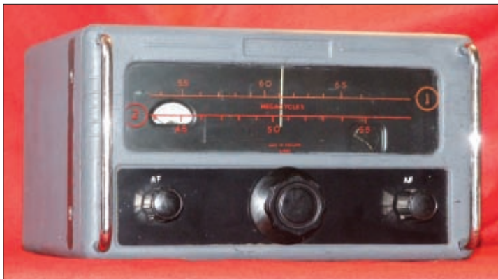
Fig. 1: The 'Special' 930 type Eddystone receiver, which was once used by the BBC for monitoring Band I (v.h.f.) 405-line TV sound transmissions.
