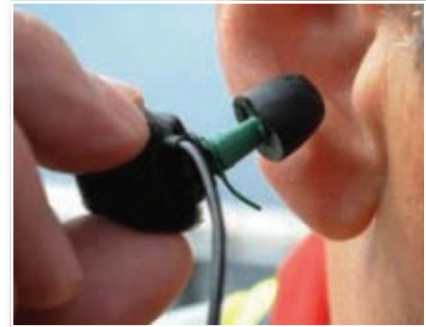
The 'Quietpro' earplug was originally developed for noisy locations. It features external sound-cancelling on the earphone and the built-in microphone.
