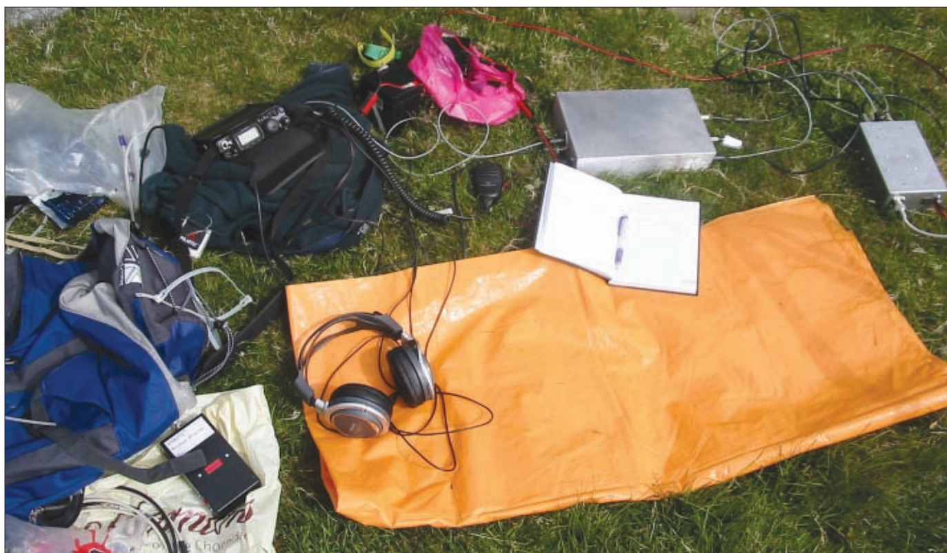
Fig. 13: The station, used for hilltop portable operation – transceiver and transverter and the essential waterproof bag that doubles as a mat for use on damp grass!
