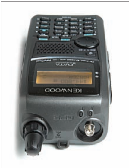
The very simple plain top with the recessed SMA antenna connection.
