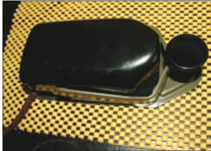
Fig. 1: The Czech Morse key seen from the outside.
