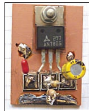
Fig. 5: Artificially increasing the regulated output voltage with two fixed value resistors.
