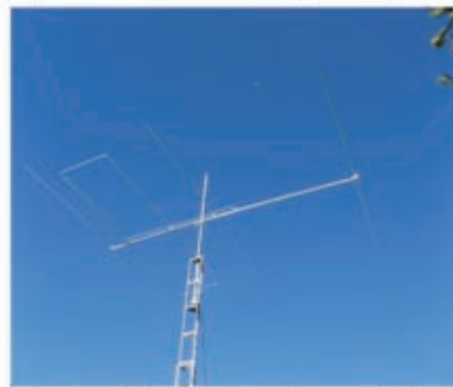
A 4 element 28MHz LFA Yagi installed at VK4NXD
