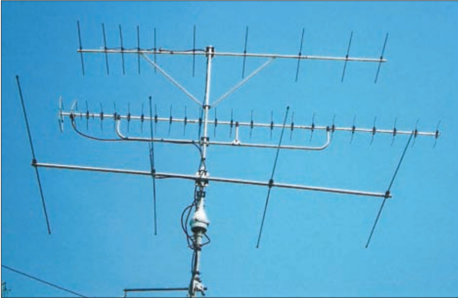
Fig. 2: From 'down-under, Steve Mahoney VK5AIM's antenna system for 50, 144 and 432MHz. Makes you jealous, doesn't it?
