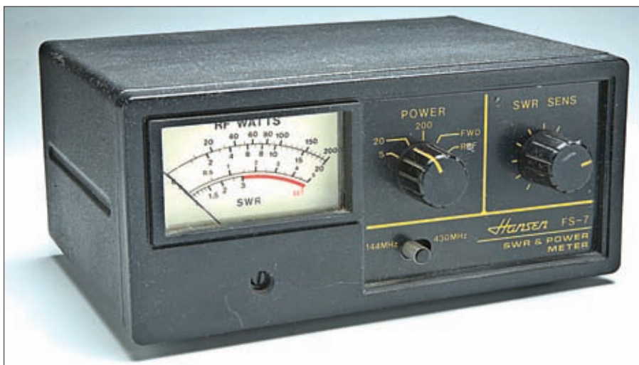
Fig. 5: A v.h.f./u.h.f. s.w.r. meter is a handy tool to check a length of coaxial cable.
