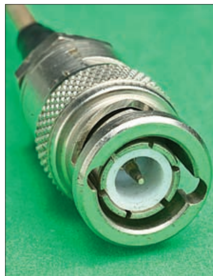
Fig. 1: A 50Ω BNC connector has its white insulator running to the end of the connector. This type when taken apart carefully, may be reused – see Fig. 2
