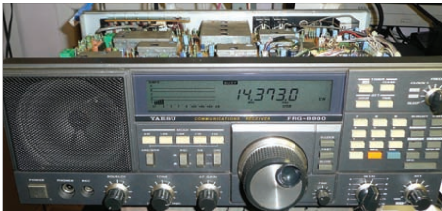
Fig. 2: The FRG-8800 was a popular general coverage receiver. It was simple to use, and could be fitted with an internal very high frequency (v.h.f.) converter, but it has a 'quirk', which Harry discusses this month.
