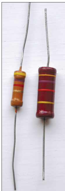
Fig. 5: Good light is needed to clearly identify resistors using their colour codes – these example are both 4.7kΩ.
