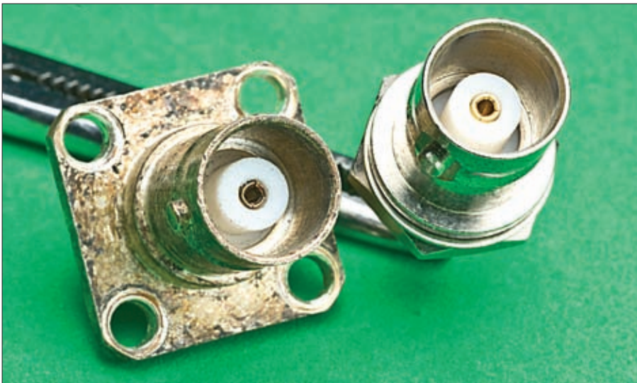
Fig. 4: Spot the difference! The 75Ω socket with its slightly smaller centre connector is on the left. The 50Ω BNC socket is on the right.
