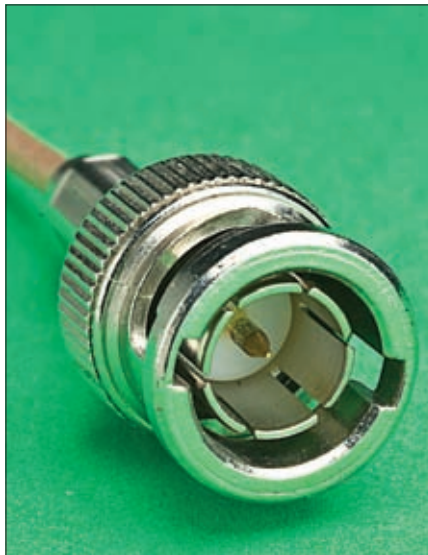
Fig. 3: Spot the difference with the lack of insulator on this 75Ω BNC plug. This type is a 'crimp-on' type and cannot be re-used.
