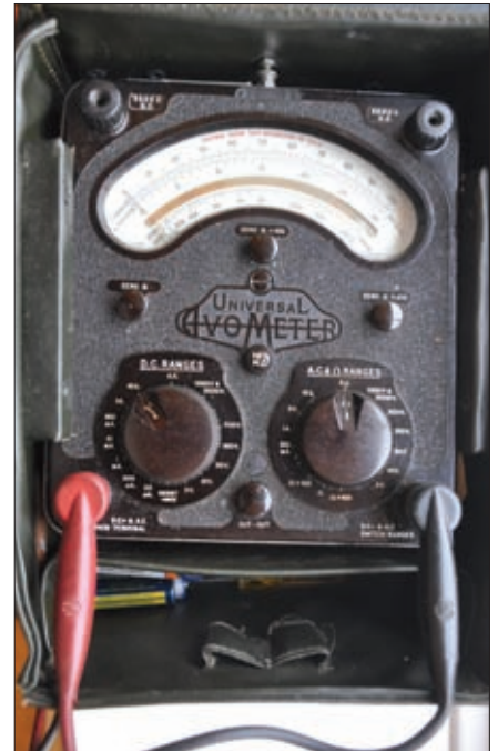
Fig. 4: Second-hand AVOs multi-meters can be picked up at rallies and last a lifetime.
