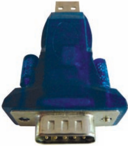
Fig. 1: A converter from USB to RS232 serial interface.
