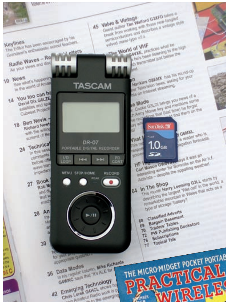
Fig. 2: With built-in stereo microphones, electronic recorders are now capable of storing several hours of CD-quality sound on small memory cards.
