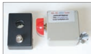
Fig. 3: The two additional boxes, Ben would have preferred the coaxial socket to have been on the bottom of the coupling box.
