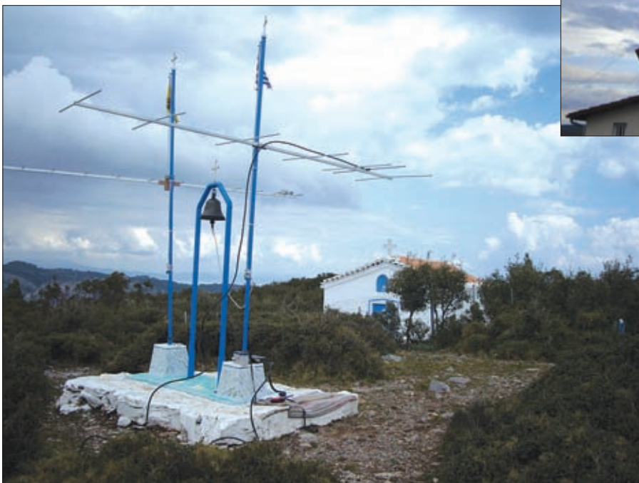
An unusual mounting point for a pair of v.h.f. antennas sent in by Panos SV1GRN who writes on behalf of the Athens QRP group.
