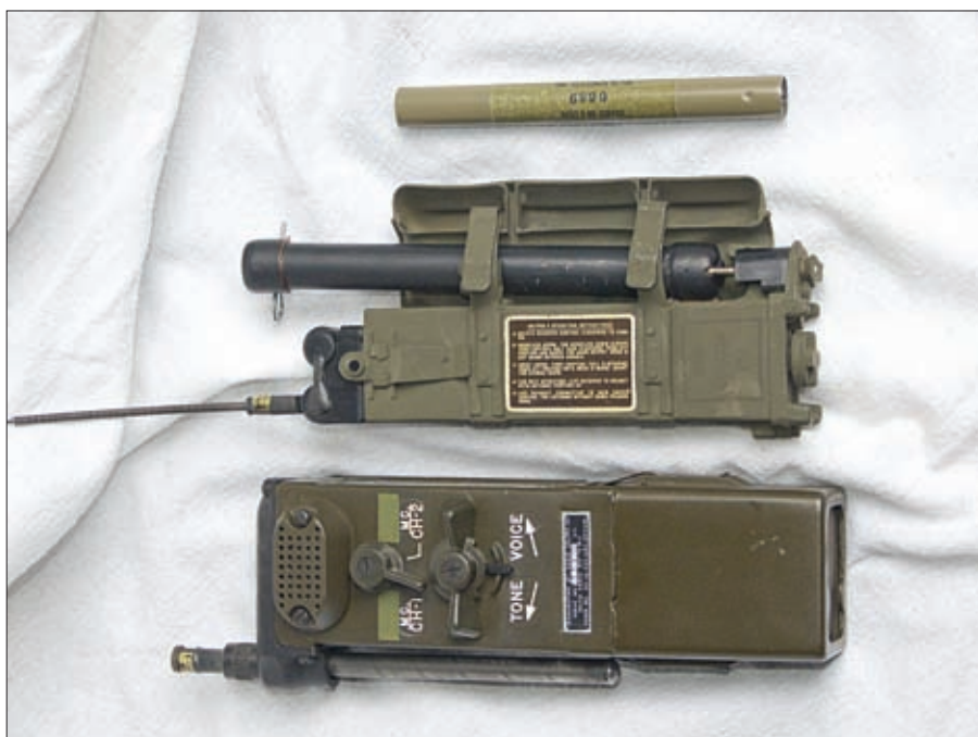
Fig 3: The PRR9 and PRT4 radio set, the original receiver battery is held in the small tube (top of photo).
