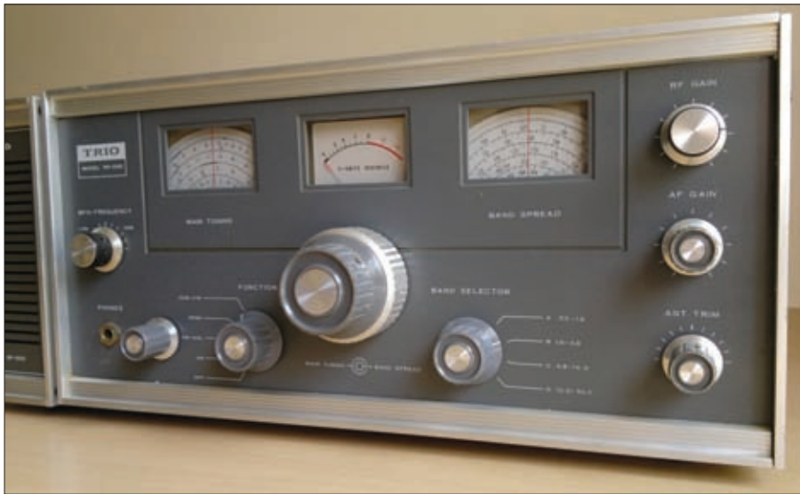
The Trio 9R-59 series of receivers, with the matching speaker alongside (partly obscured in this view), can still hold its own against some more modern sets. The dual concentric tuning controls. The rear section for the main tuning (left-hand scale), the front knob controls the band-spread (fine tune) of the right-hand dial.
