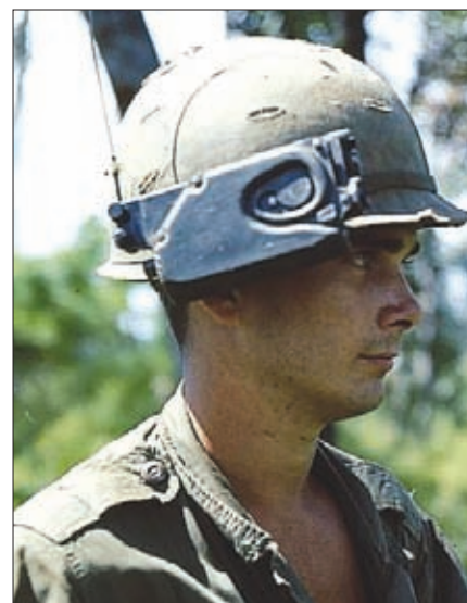
Fig 3: The PRR9 and PRT4 radio set, the original receiver battery is held in the small tube (top of photo).
