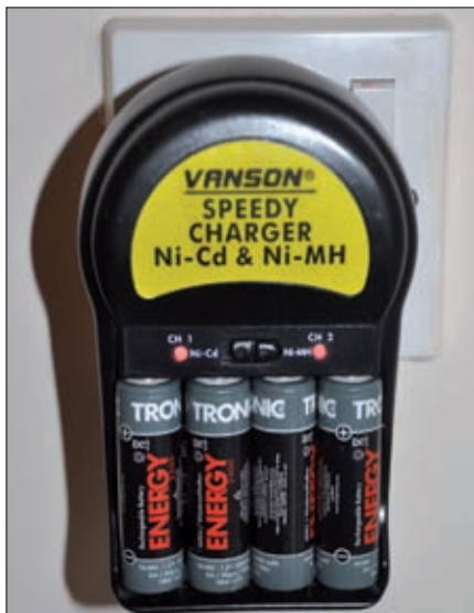
Fig. 3: A charger for size AA batteries. There's a switch to select between Ni-Cad (constant current charging) and Lithium Metal Hydride (constant voltage charging) batteries.
