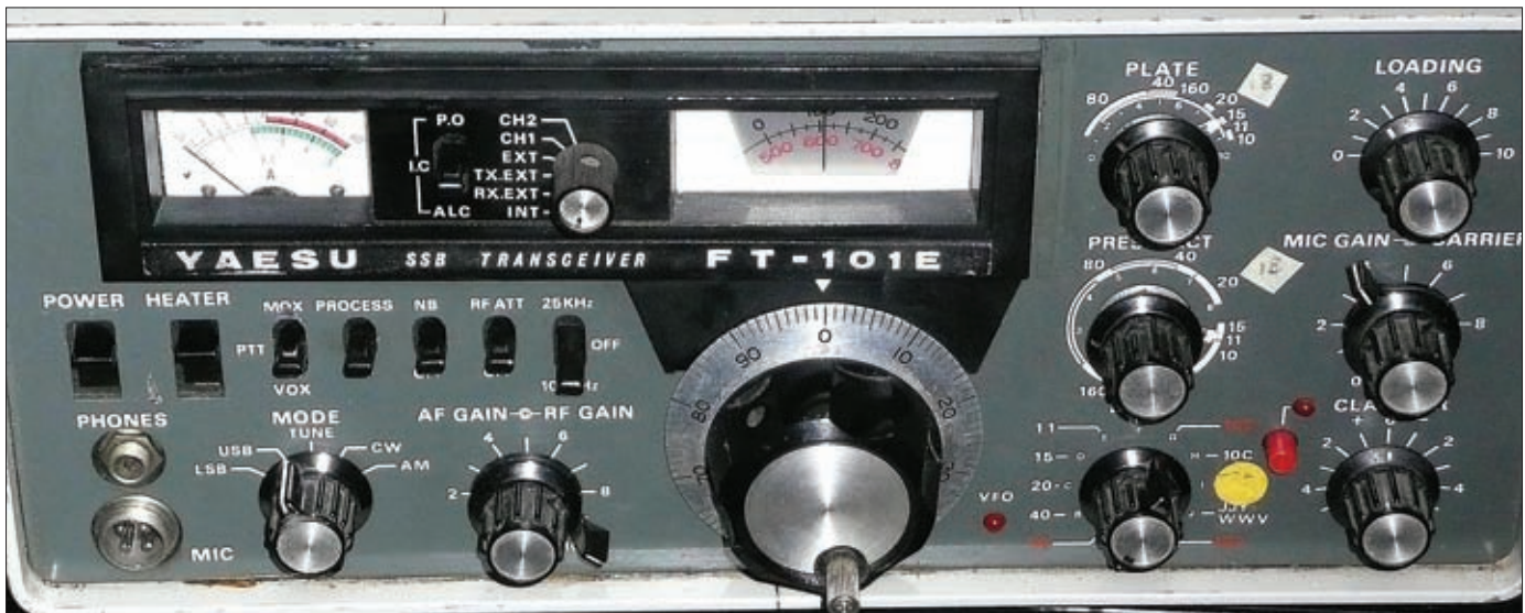
This is an early version of the FT-101. How can we tell? In later models, the Clarifier control (bottom right) has become a dual-concentric control with the speech compressor control on the rearward portion.
