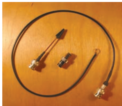
Fig. 8: Accessories – a short antenna and an inductive pick-up loop for sniffing along tracks on a circuit board.
