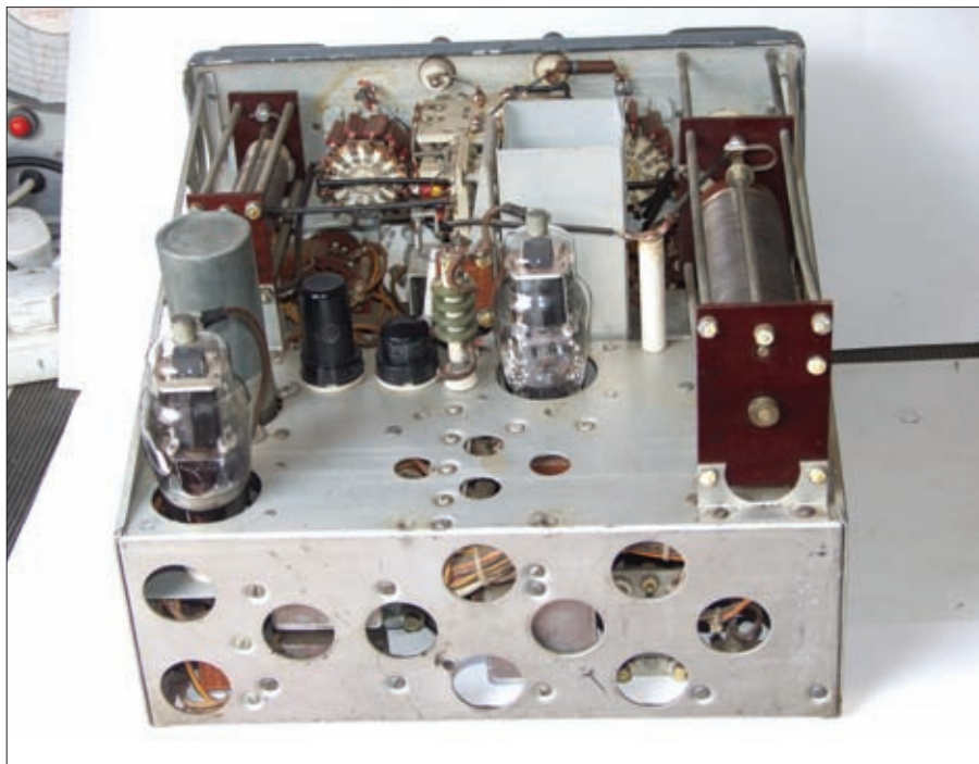
Fig 2: Internals of the AT1, the space in the centre is where the dynamotor, changing the incoming 12V up to 500V, is normally located.
