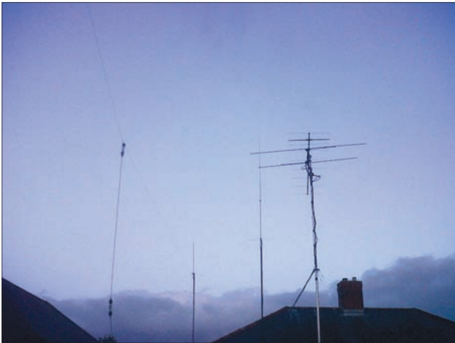
Along with the two horizontal v.h.f. arrays, and the multi-band vertical at 2W0ZJA, there's a CWS-80 Carolina Windom for h.f. too.
