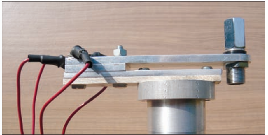
Fig. 5: Dave's answer to the problem was to add an insulating 'washer' under the bracket, so separating the bracket and metal pole.
