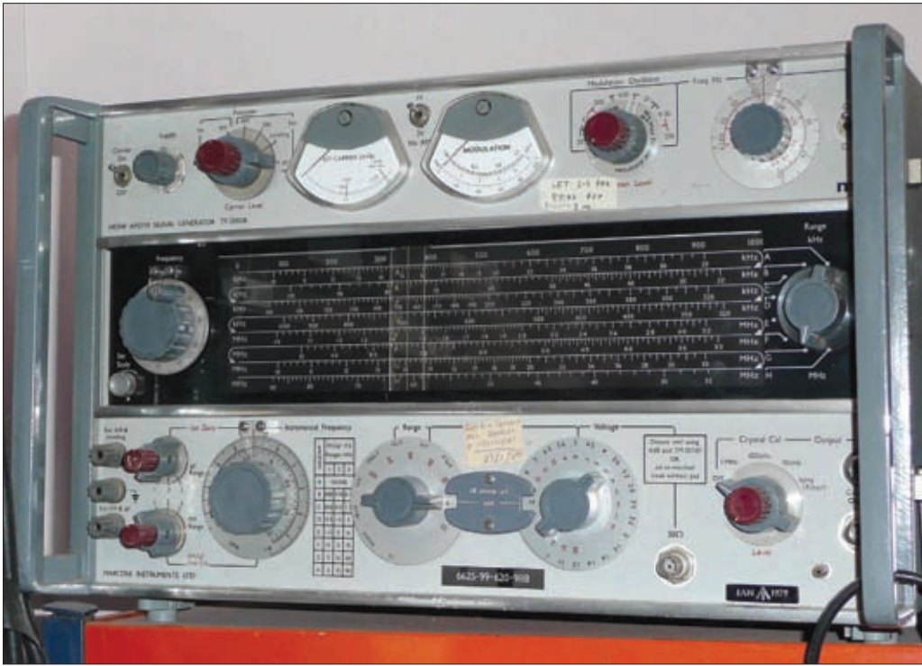
Fig. 2: Big it may be, but the internal screening of this Marconi TF202B at nearly 50 years old, is very good, making it possible to inject low level signals into a receiver without swamping it.
