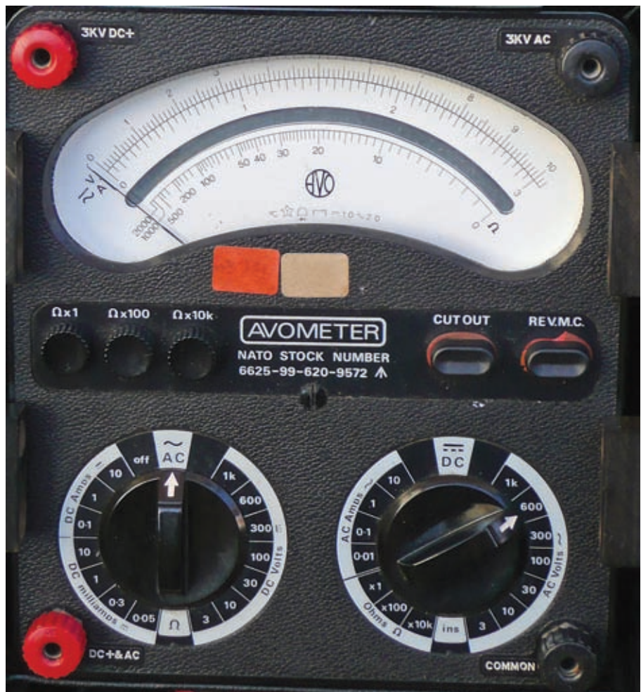
Fig. 3: Not only was the AVO Mk8 multi-meter a fine example of measuring equipment, but its statement of accuracy was explicit too! Unlike many items that come up for sale.
