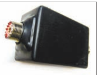
Fig. 2: The supplied UNUN has one end colour-coded to enable it to be fitted the correct way round.
