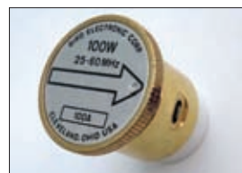
Fig. 3: Just one example of the rotatable sensing elements available for the Bird Thru-line. This one is suitable for frequencies of between 25 and 60MHz, with powers up to maximum of 100W. Other combinations are available.
