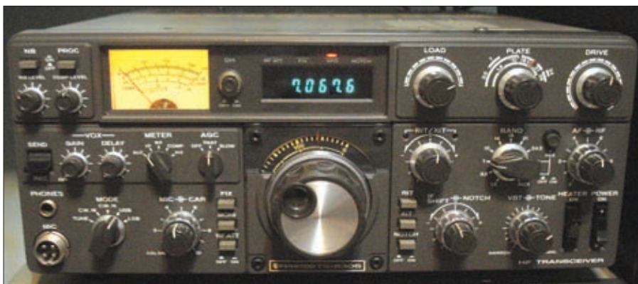
Fig 1: Kenwood's TS-830 h.f. transceiver with a valve power-amplifier was a highly regarded transceiver in the 1980s.
