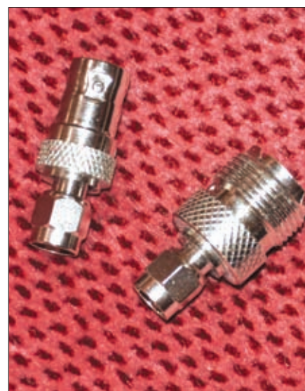
Fig 3: Adaptors to allow modern hand-held transceivers with SMA antenna sockets to be used with feeder terminated in BNC (left) and PL259 (right) plugs.
