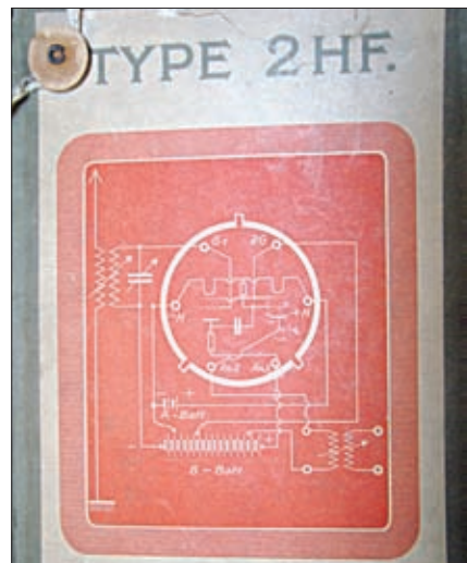
The information sheet for the 2HF, a two-unit valve designed for r.f. use.
