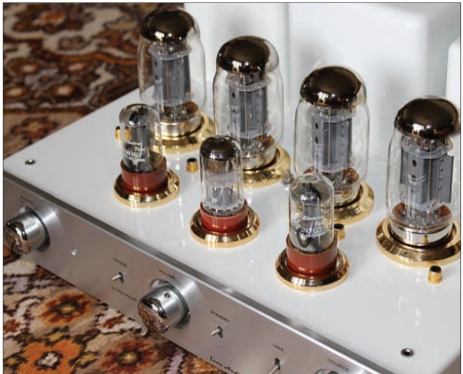
Fig. 6: A modern 50W per channel valved amplifier from Icon Audio. The low-level valves are 6SL7GT (centre, and higher \mu than the 6SN7) flanked by two 6SN7GT phase splitters. The output valves are four KT88s, switchable between triode and ultra-linear connection.
