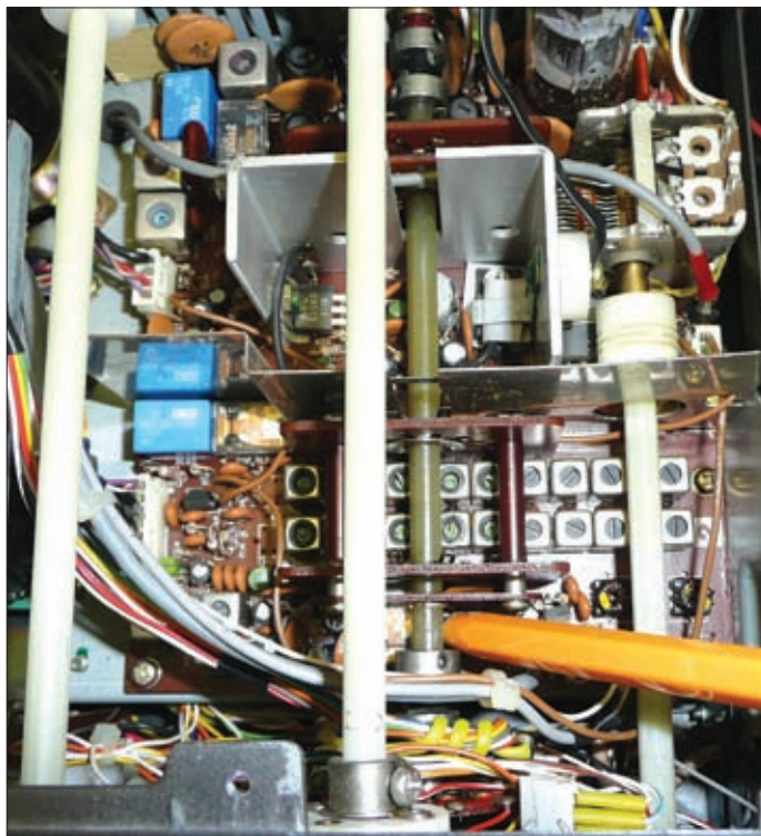
Fig. 2: The r.f. board from the FT-102. Note that there's a reflection of the lower blue relay on the metal screening wall. Once you've removed the relay covers you will need some switch cleaner that does not contain a lubricant.
