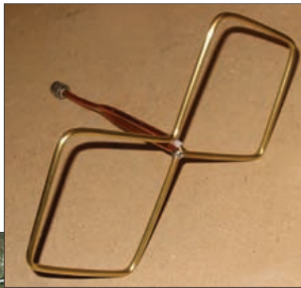
Fig. 6: The 'bi-quad' as constructed.
