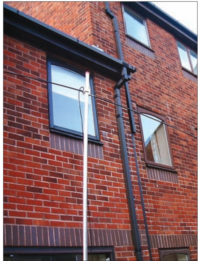
Fig. 4: Two mobile whips fitted back to back to form a dipole with coils to reduce the dimensions to a fraction of a normal dipole length.
