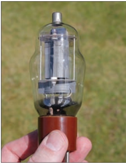
Fig. 3. An 807 – maker unknown. The electrode structure is similar to that of the Brimar 6L6GA. Notice the screen around the lead-out wires to minimise coupling between the anode and the control grid.
