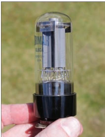
Fig. 1: Brimar's 6L6GA, a recent glass tubular version of the original metal 6L6.
