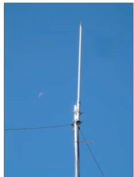
Fig. 2: A small triple-band (50/145/433MHz) antenna, which is ideal for local contacts. Notice how the support mast has also been used to support the feed-point of a wire antenna saving the visual impact of a second support.
