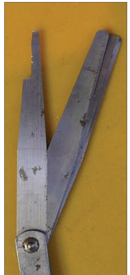
Fig. 4: Feeler gauges can make an ideal relay contact cleaning tool.
