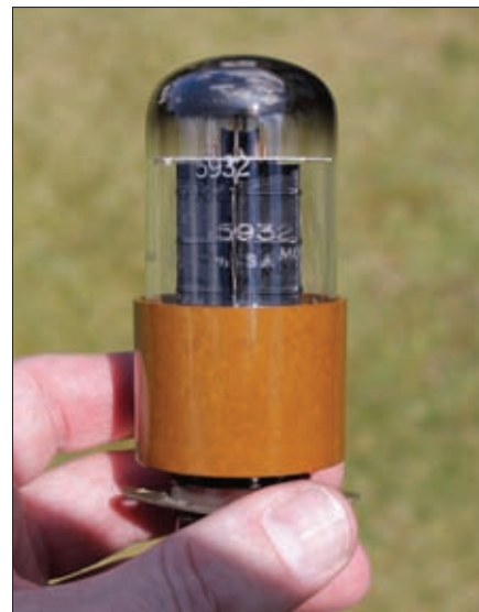
Fig. 2: A ruggedised version of the 6L6G, the 5962/6L6WGA produced by Sylvania.
