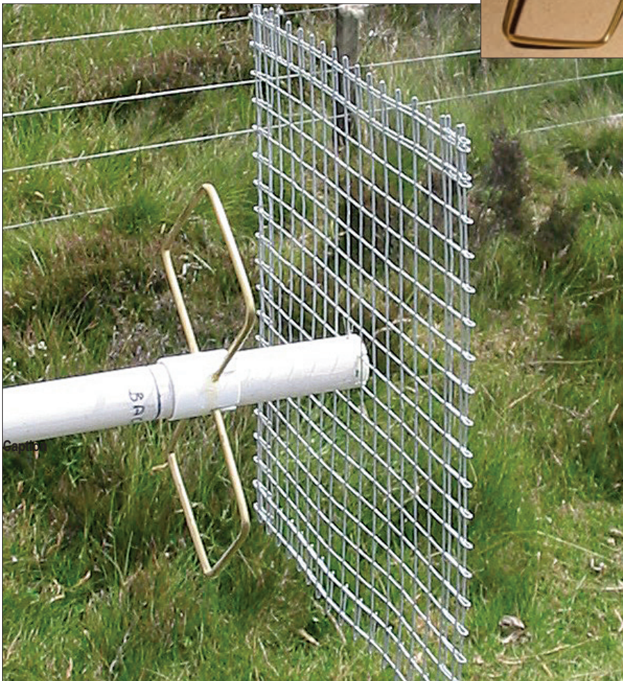
Fig. 6: The 'bi-quad' as constructed.
