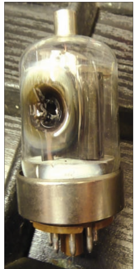
Fig. 3: In spite of their thermal robustness, valves can actually melt with the heat generated.
