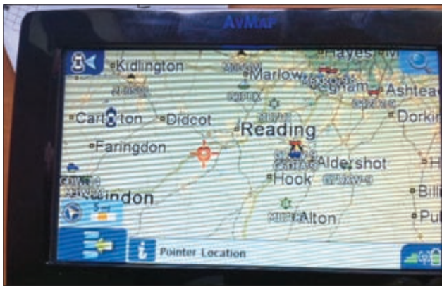
Two photographs of the Avmap Geosat 6 APRS unit's screen in operation. The banding shown on the screen is a problem of taking a photograph, rather than a problem with the screen itself.
