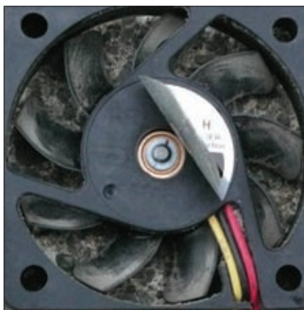
Harry found that peeling back the label on a fan motor and squirting some lubricant into the bearings, helped the fan to run freely.
