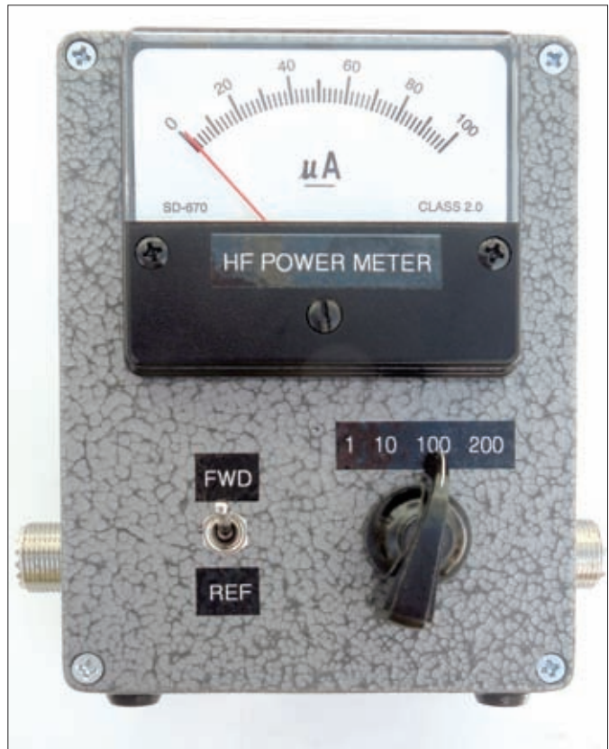
The prototype unit in its smart grey Hammerrite finish die-cast box. The power scale wasn't calibrated at the time this picture was taken.
