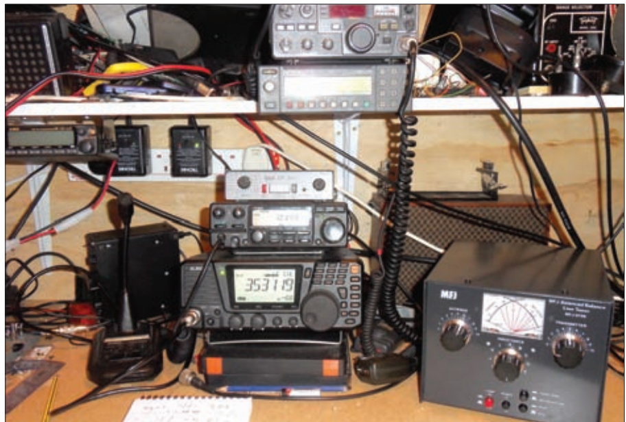
Fig. 1: The MFJ-974B in Rob G3XFD's shack (to the right of the Alinco DX-SR8 transceiver) where he found it out-performed his MFJ roller coaster a.t.u. when it was being used with a balanced feeder antenna.
