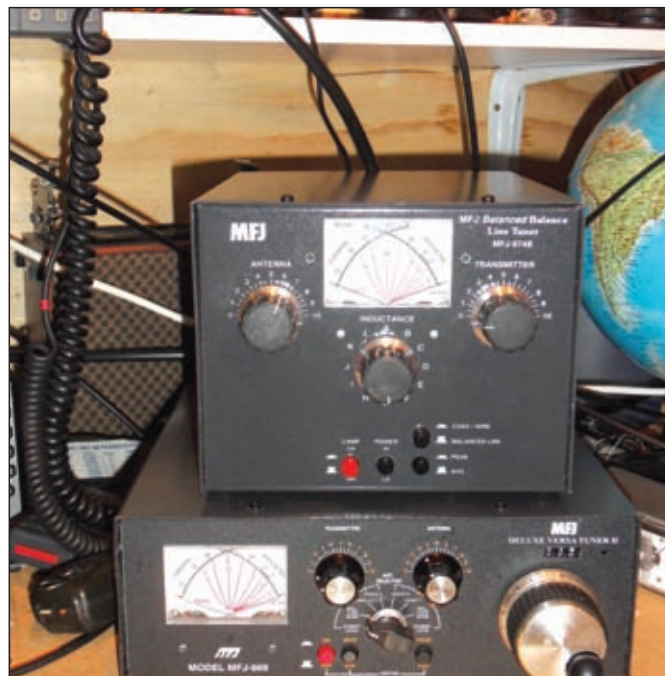
Fig. 2: Close up view of the MFJ-974B perched on top of it sibling MFJ Deluxe Versatuner II. Rob found the single large rotary switch of the balanced tuner, that selects theappings on the inductor – to be more convenient.
