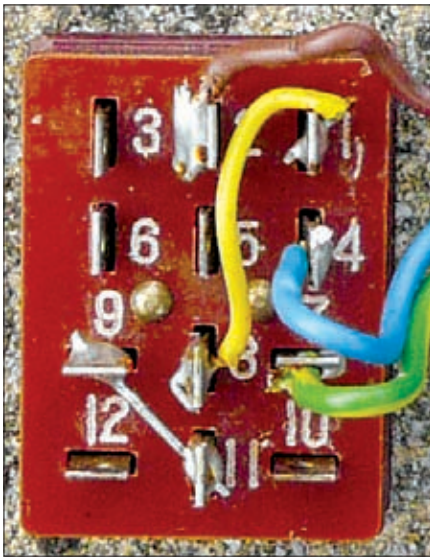
Fig. 3: The mains connector for the B and E versions of the FT-101MK1.
