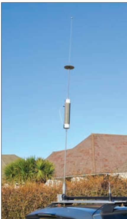
Fig. 1: The Texas Bugcatcher antenna mounted on the rear of an estate car.
