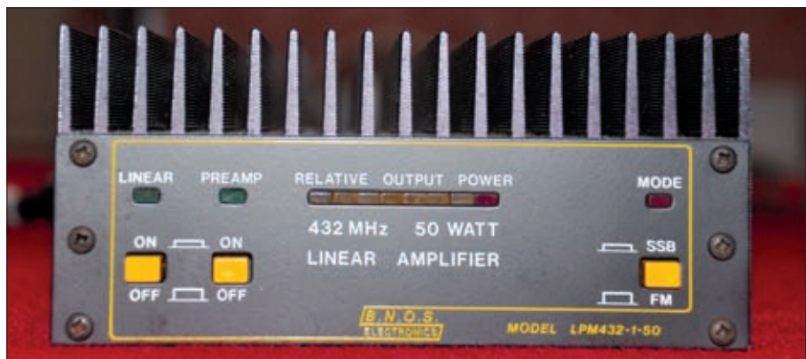
Fig. 4: A combined pre-amp and power amplifier designed for 1W input power on 432MHz. Note the f.m./s.s.b. switch on the bottom right. This control determines whether there is a delay in switching back from transmit to receive when r.f. sensed switching is employed with s.s.b. signals.
