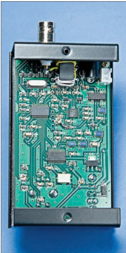
Fig. 1: Inside the YouKits FG-01 SWR Analyser, as you'd expect with such a small unit, it's mainly surface mount components.
