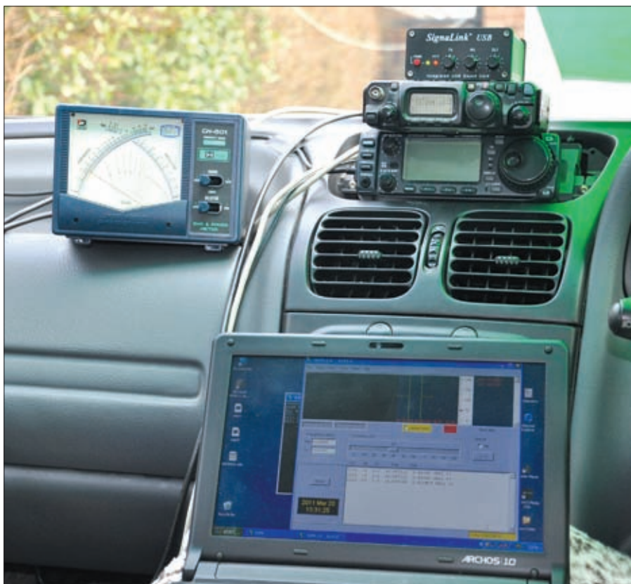
Fig. 3: The WSPR test setup using the FT-817 with Signalink USB interface perched on top of the normal mobile remote box (not used in this test).
