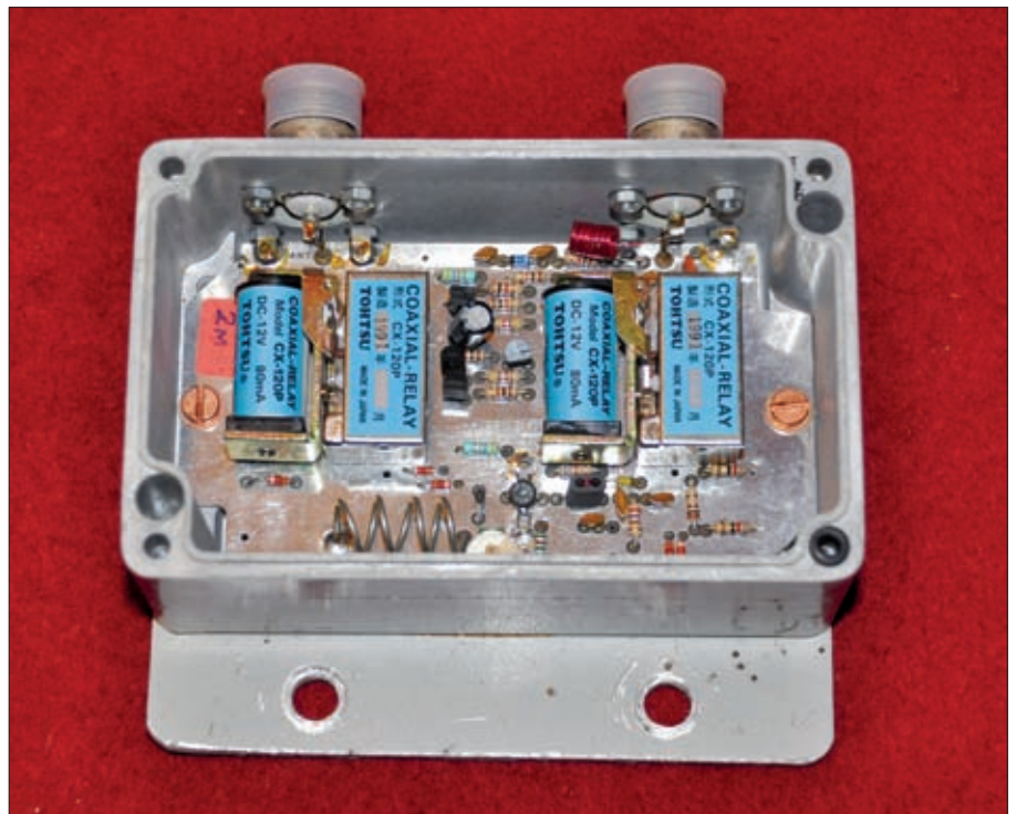
Fig. 2: A waterproof pre-amp designed for mounting at the masthead. The p.c.b. mounted input and output relays are clearly visible.
