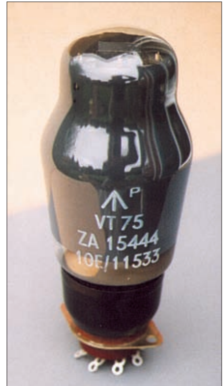
The military version of the KT66 with its shrouded glass envelope, made it difficult to see what configuration the valve had. Contrast this with the 'civilian' version in the other photograph!
