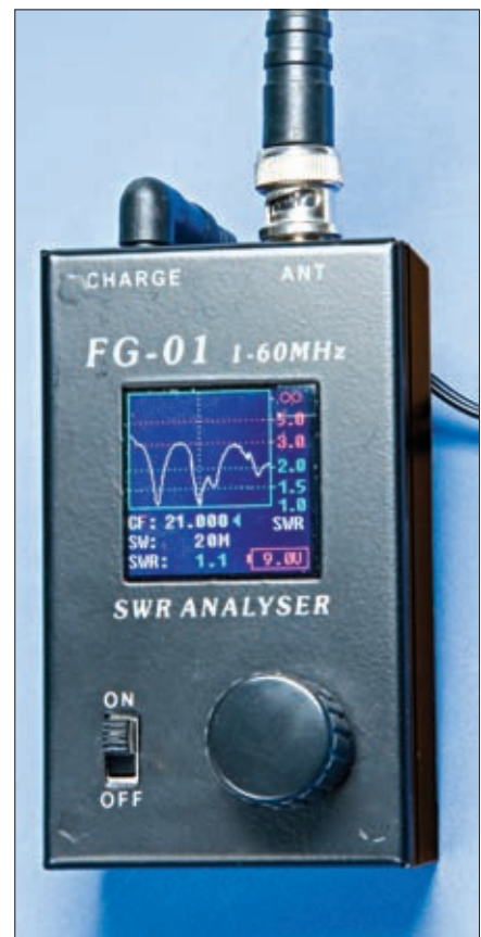
The YouKits FG-01 SWR analyser showing the variation of s.w.r. to be found in a typical multi-band antenna.
