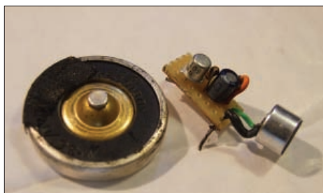
Fig. 2: The Electret replacement amplifier (right) built by Ben G4BXD using Veroboard.
