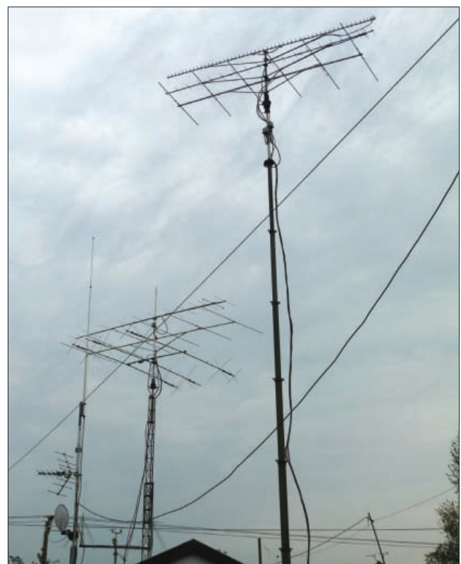
Fig. 2: The antennas at Andy GM4JR's station. The 6-element 70MHz antenna is the lowest on the mast nearest the camera with a 21-element Yagi for 432MHz and a 55-element Yagi for 1296MHz above it.
