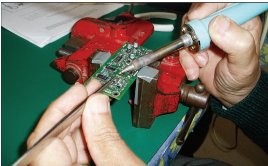
Phil's method of working on the surface mount board of the Finningley SDR kit.
