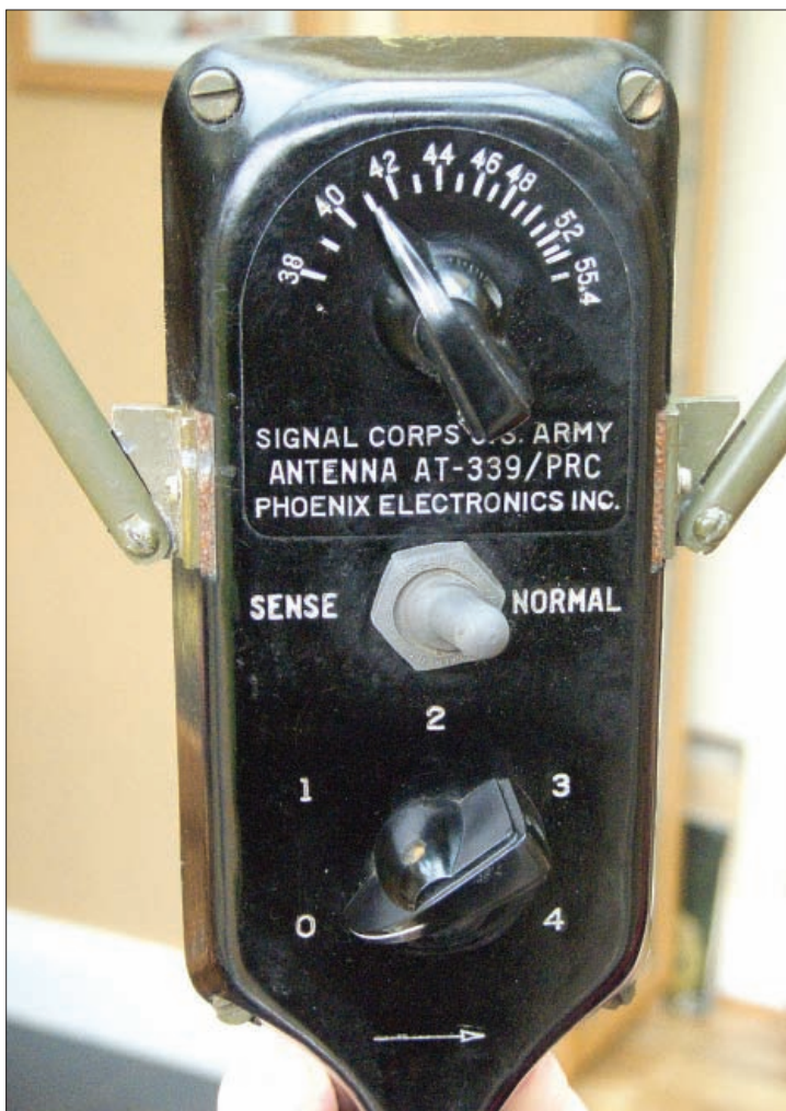
Fig. 5: Close-up view of the controls of the hand-held loop.
