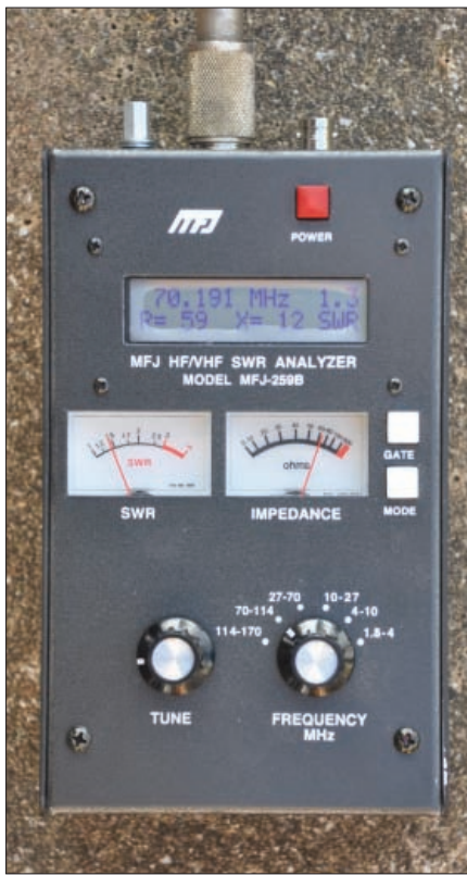
Fig. 5: Measurements of the s.w.r. of the 70MHz Yagi using an MFJ-259B Antenna Analyser.
