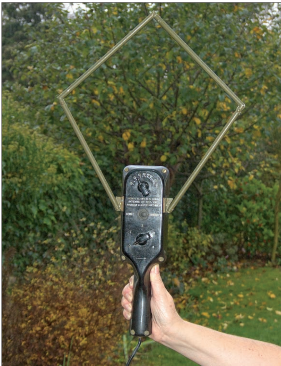
Fig. 4: The hand-held loop antenna – with it, Ben located a nearby baby alarm on 49MHz!
