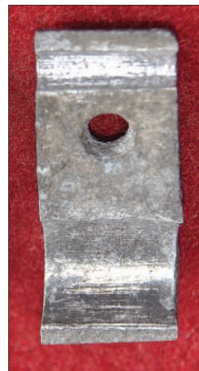
Fig. 4: Corrosion on the end of the matching rod – before cleaning (left), and after cleaning (right).
