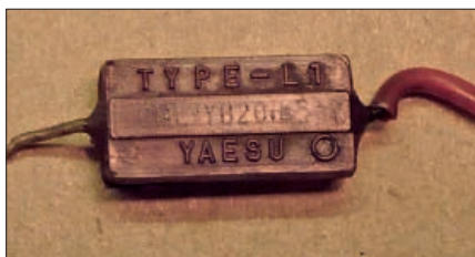
Fig. 2: This capacitor could be well past its 'use by' date, better to check carefully before using it.
