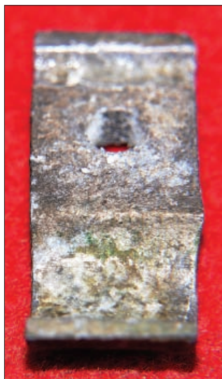
Fig. 4: Corrosion on the end of the matching rod – before cleaning (left), and after cleaning (right).
