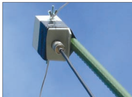
Fig. 2: a closer look at the bottom of the 1:4 step-up balun, which Ray bought some time ago before they went up in price significantly.
