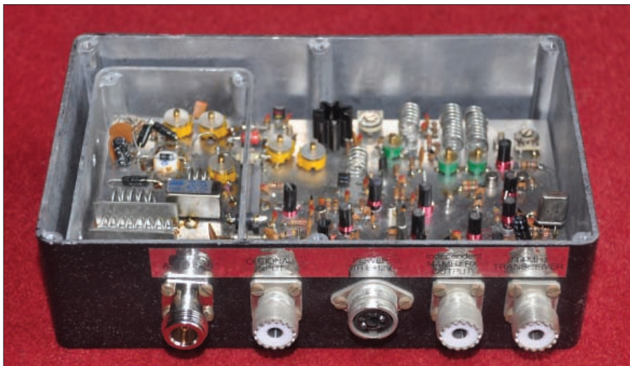
Fig. 1: The Microwave Modules transverter with the N-socket from Rapid Electronics mounted on the left, replacing the original BNC socket for 70MHz.
