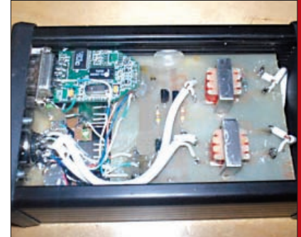
Fig. 7: The p.t.t./c.w. circuit and isolation transformer.
