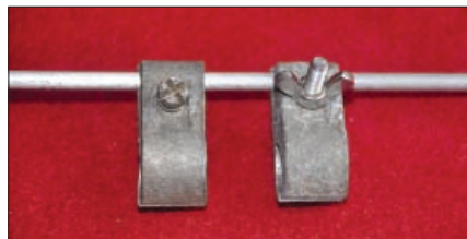
Fig. 2: The M5 screw and wing nut (on the right) used by Colin alongside the old Tonna screw arrangement (on the left).
