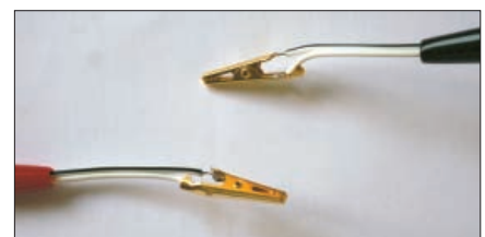
Fig. 2: The physical form of the four-wire connections to test clips.
