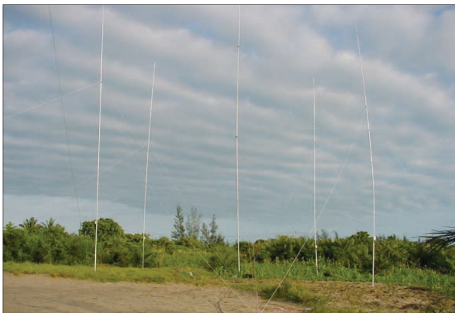
Fig. 2: The 7MHz 4 square antenna used by Daniel Hubbard when he was operating as C91JR.
