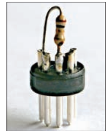
Fig. 8: The internal view of the 1Ω resistor mounted directly onto the pins of the plug.
