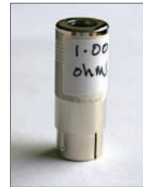
Fig. 7: The 'One ohm in a plug' which Colin uses as a standard value for testing and setting up.
