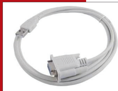
Fig. 4: A USB-to-serial adapter. But beware of some cheap versions available from eBay – they have a high failure rate.
