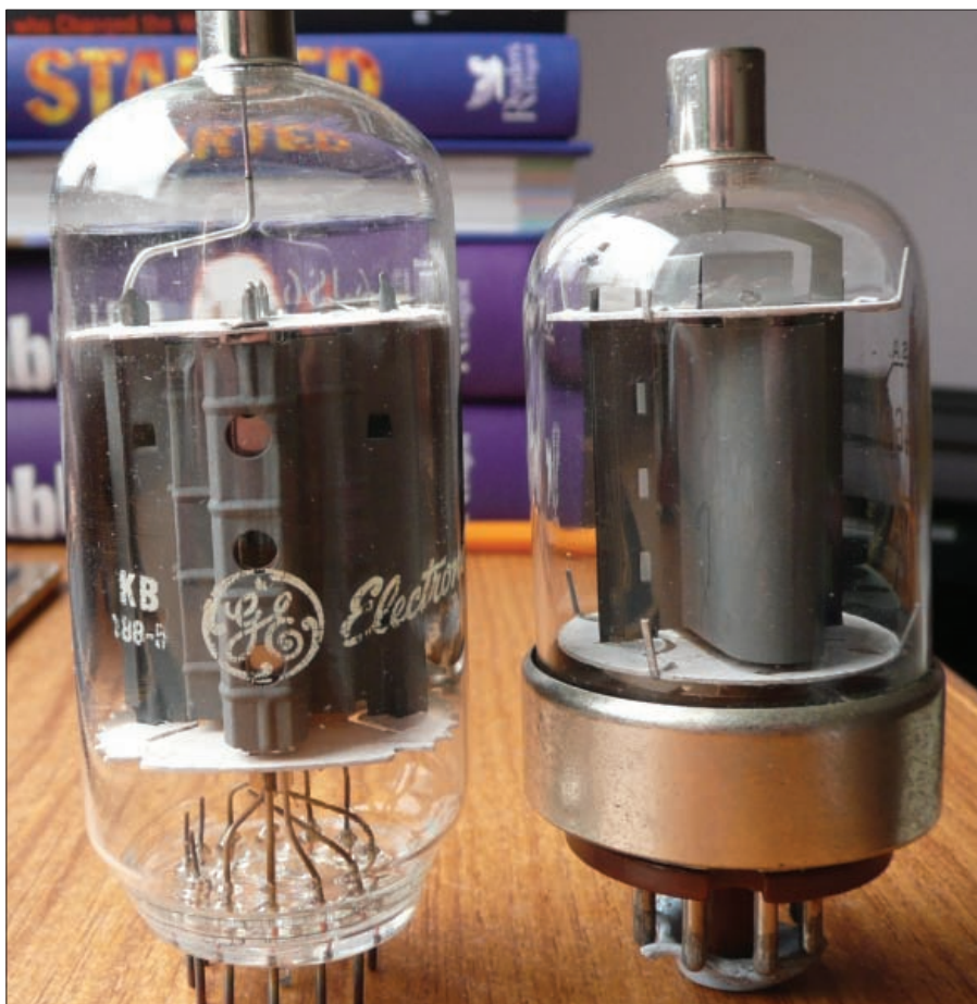
Spot the differences and similarities. Construction of the line output valve (on the left) is very similar to the 6146 power amplifier valve on the right.
