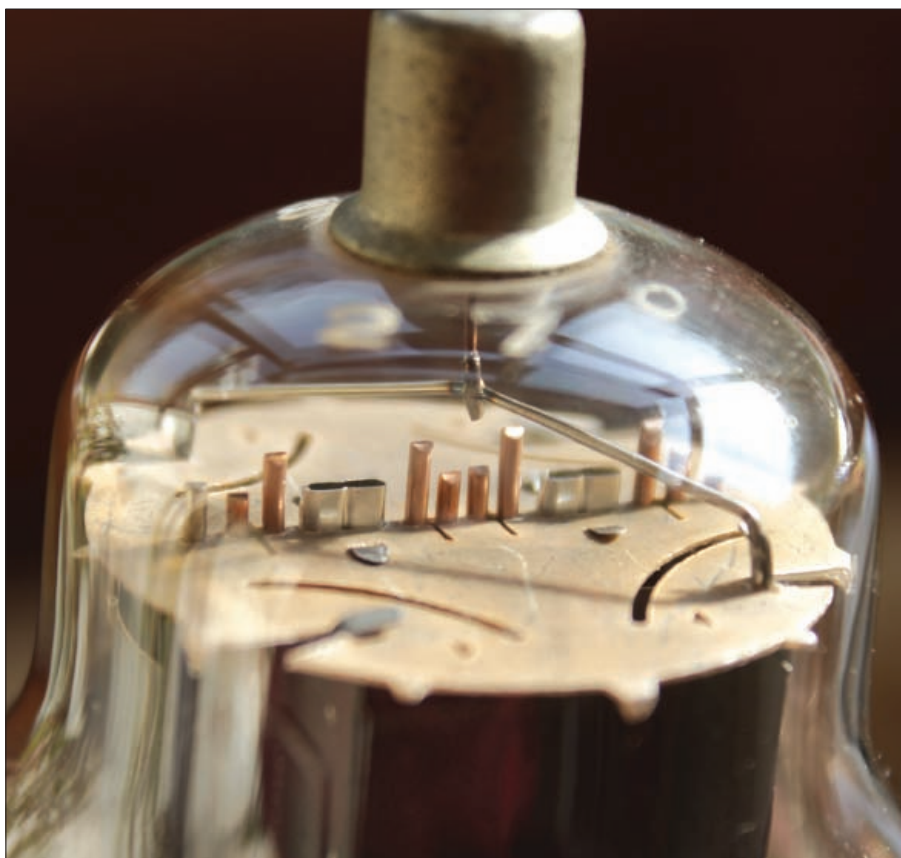
Fig. 3: Looking at the electrode tops of a 6CD6G line output valve which has twin cathodes and twin electrode structures and is very similar to a KT55 valve.
