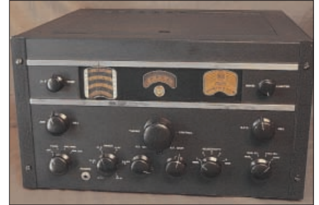
Fig. 4: Still a good radio, in spite of its weight – the war-time vintage AR88 receiver.
