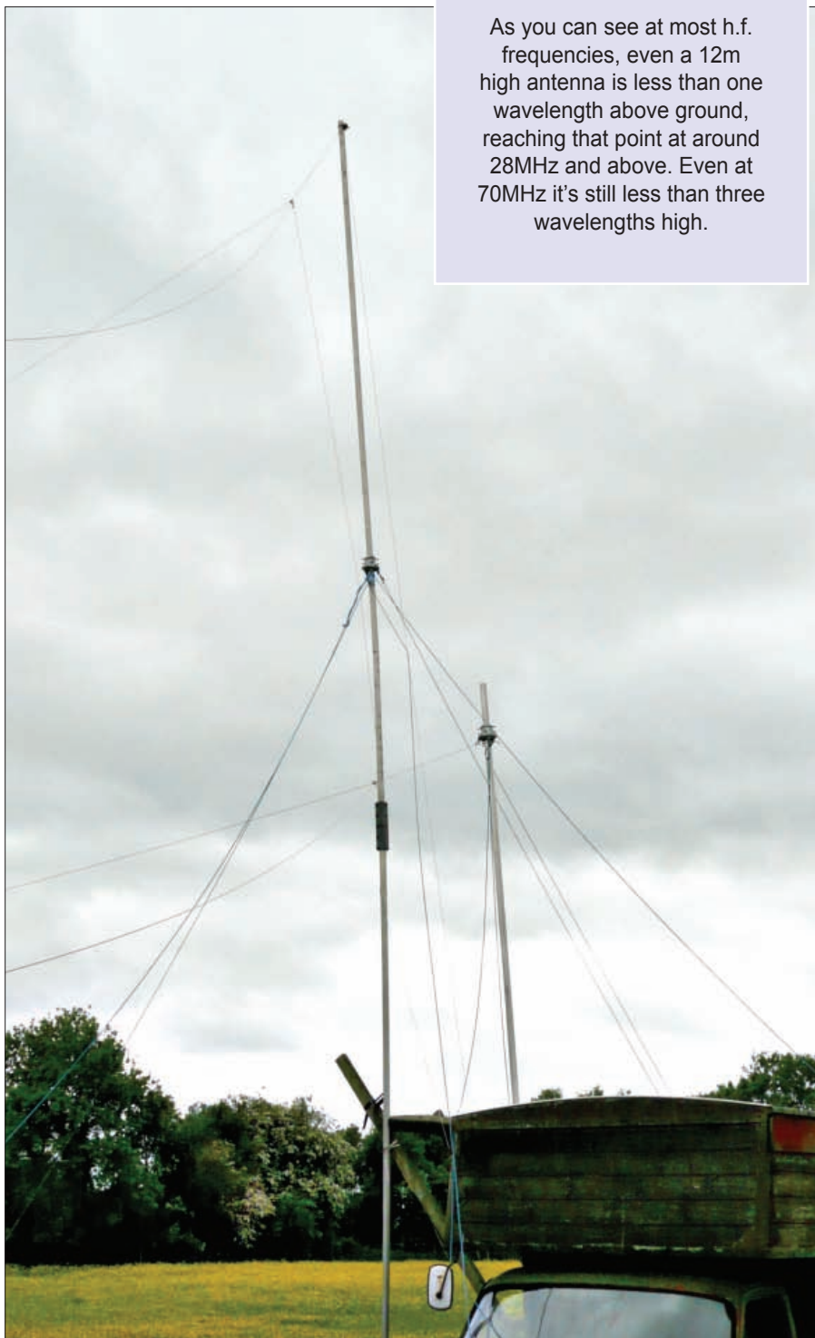
Fig. 5: Ian G3WRT has used a reduced stay system for some time now, utilising the tension in the antenna wire as one of the supporting tensioners. Not ideal perhaps, but it does work!
