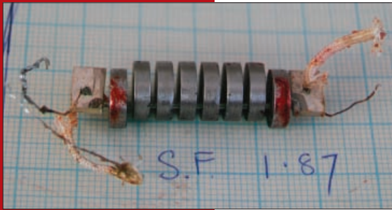
Fig. 8: The filter itself, after cleaning, ready for remounting.
