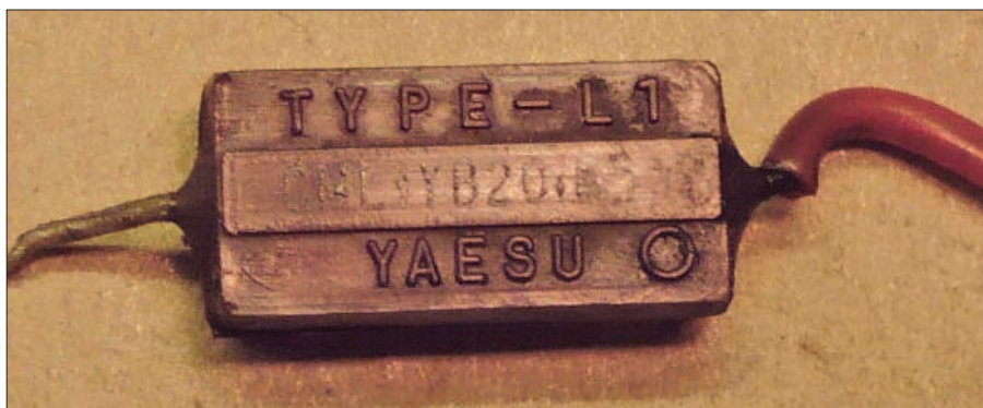
Fig. 2: The suspect capacitor with Yaesu markings.
