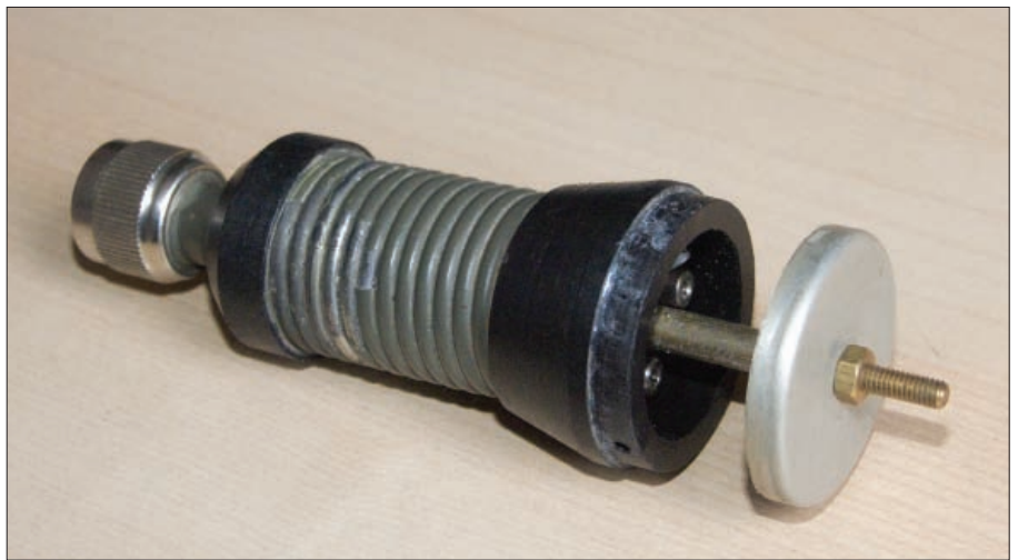
Fig. 2: The airband antenna internally – it seems to be just a disc. If you can help Ben with information on this antenna he would like to hear from you.
