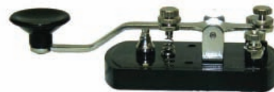
Fig.10: The MFJ 5501 Morse key used by Geoffrey M1EDF.
