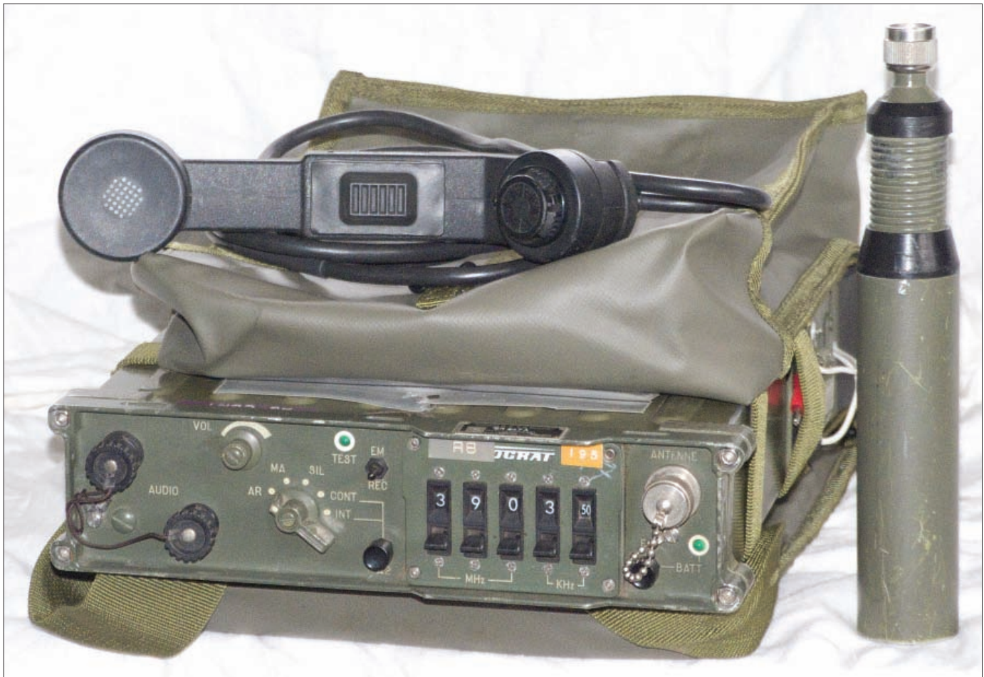
Fig. 1: The u.h.f. airband transceiver (note the odd antenna on the right).
