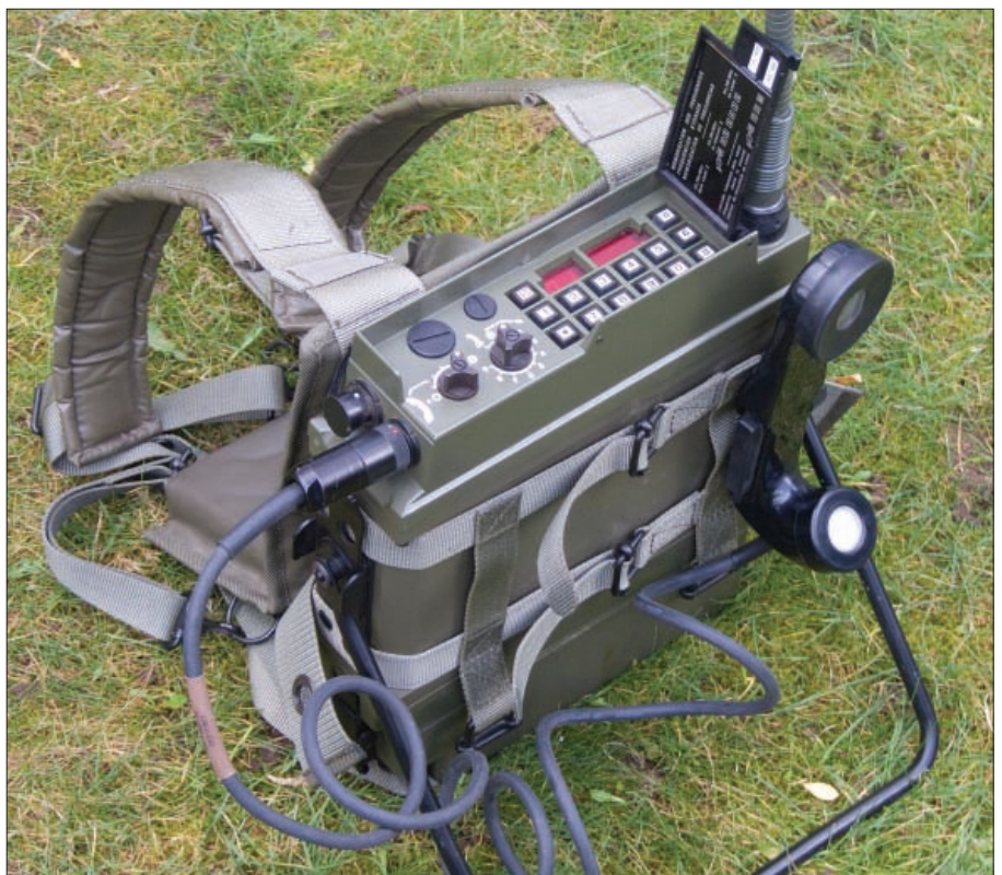
Fig. 4: The French TRC-552 v.h.f. transceiver.
