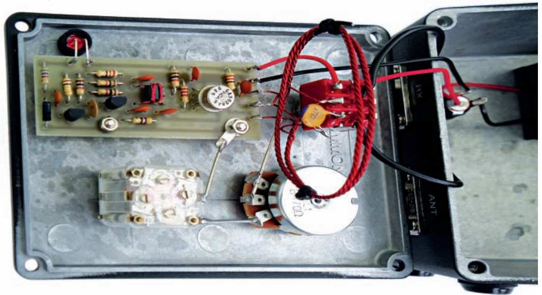
Fig. 5: The circuit boards as fitted into the finished project box.
