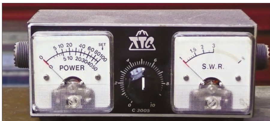
Fig. 5: A simple two-meter s.w.r. meter, indicates the power going forward towards the antenna on the left hand meter, and the reflected power from the antenna on the right hand meter, which is scaled in s.w.r.
