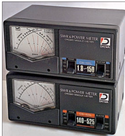
Fig. 2: A 'cross needle' type of s.w.r. meter.
