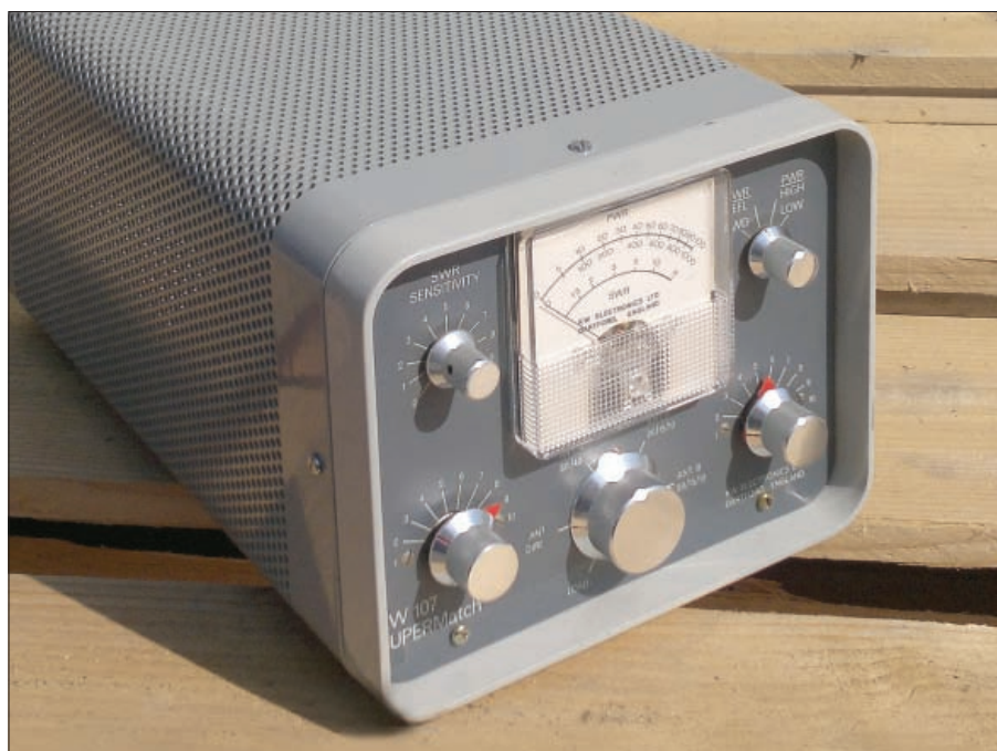
Fig. 5: A KW107 antenna matching unit – a very popular and 'long lived' unit.
