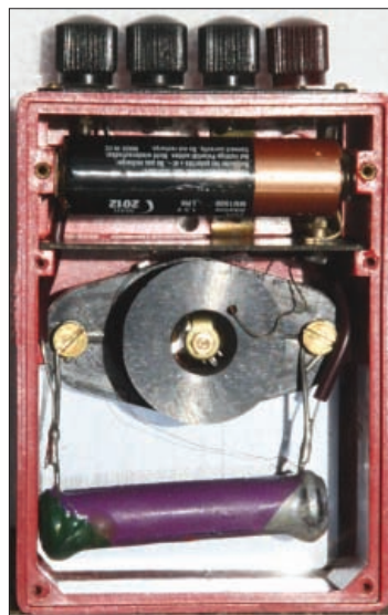
Fig. 4: This internal view is dominated by a carbon-composition resistor (bottom).
