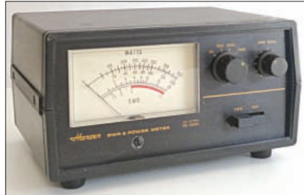
Fig. 1: An s.w.r. meter designed for Amateur Radio use.
