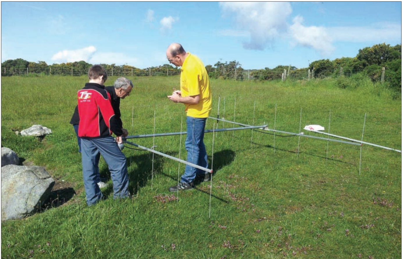
Fig. 2: The Isle of Man Amateur Radio Society's joined in during the Practical Wireless 144MHz QRP contest. They operated from the village of Ballaragh (east coast of IOM). The antennas were a pair of stacked 9-element Yagis constructed from the remnants of some scrap Tonna antennas and these are being assembled in the photo.
