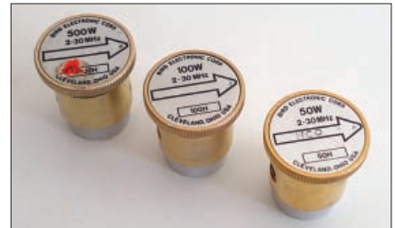
Fig. 4: Bird sensing elements – these are important and Chris G4HCL offers important advice in the article.
