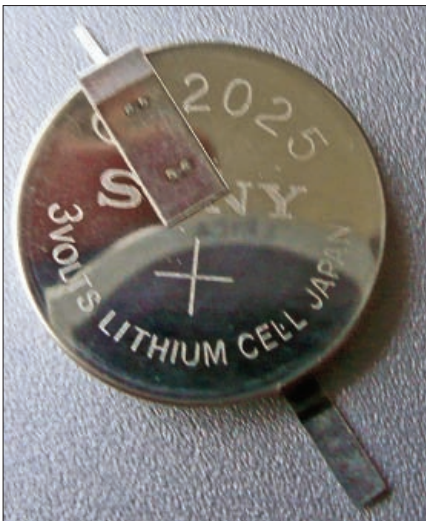
Fig. 1: The original battery on the Yaesu FT-290 Mk1 is fitted with solder tags.
