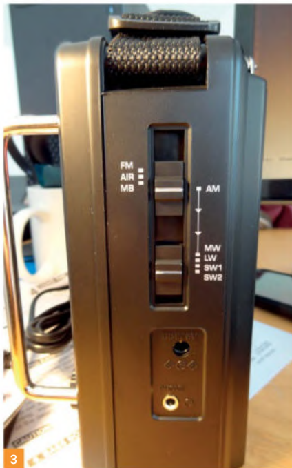
Fig. 1: The front of the (larger) Steepletone MBR1051. Fig. 2: The frequency coverage offered by the Steepletone MBR1051. Fig. 3: The simple band controls on the side of the Steepletone MBR1051. Fig. 4: A external adapter for a telescopic antenna. This may improve reception at times. Fig. 5: The Moonraker GA450 or a similar small loop can bring some signal gain. Fig. 6: The Steepletone SAB2019 and travel pouch. Fig. 7: The front of the Steepletone SAB2019. Fig. 8: Deploy a mobile phone stand to get the telescopic antenna into a vertical position and for additional stability. Fig. 9: A small active loudspeaker will improve the sound considerably. This is the Sony SRS-XB12.
