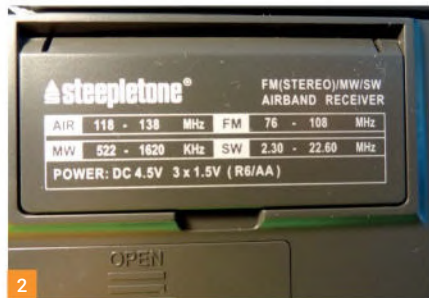
Fig. 1: The front of the (larger) Steepletone MBR1051. Fig. 2: The frequency coverage offered by the Steepletone MBR1051. Fig. 3: The simple band controls on the side of the Steepletone MBR1051. Fig. 4: A external adapter for a telescopic antenna. This may improve reception at times. Fig. 5: The Moonraker GA450 or a similar small loop can bring some signal gain. Fig. 6: The Steepletone SAB2019 and travel pouch. Fig. 7: The front of the Steepletone SAB2019. Fig. 8: Deploy a mobile phone stand to get the telescopic antenna into a vertical position and for additional stability. Fig. 9: A small active loudspeaker will improve the sound considerably. This is the Sony SRS-XB12.
