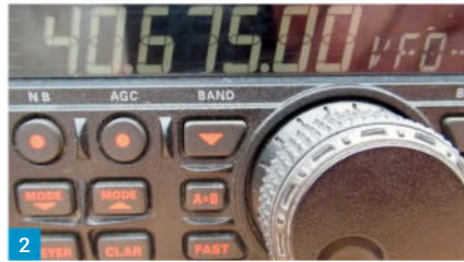
Fig. 1: The WSPRlite-Config program, compiled to cover 40MHz. Fig. 2: Kevin ZB2GI received ZS6WAB using his FT-450 on 40.675MHz.
