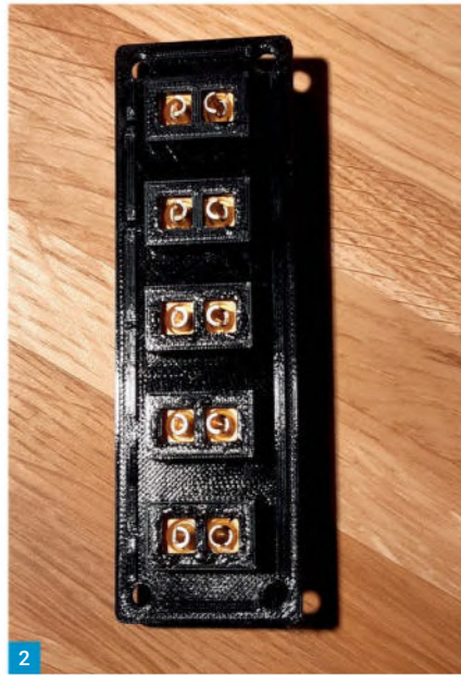
Fig. 1: An XT60 connector. Fig. 2: Male plugs glued in place. Fig. 3: Top view of glued connectors. Fig. 4: Completed daisy chained board. Fig. 5: A completed box. Fig. 6: The completed box with labelled connections. Fig. 7: The end result in the author's shack.
