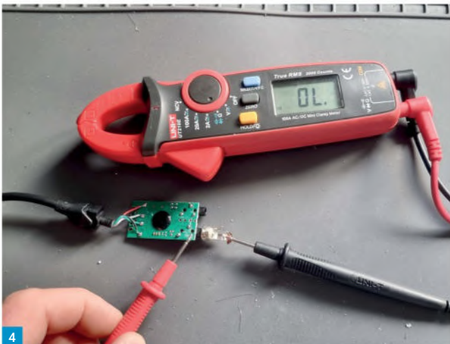
Fig. 1: The parts needed for the project. Fig. 2: Open up the soundcard PCB. Fig. 3: The transformers in place on the board. Fig. 4: Identifying the solder points on the soundcard. Fig. 5: Underside of board. Fig. 6: Connections on top of board. Fig. 7: Attaching the wires for the speaker. Fig. 8: Pin connections for the min-DIN. Fig. 9: The three connections as described in the text. Fig. 10: The completed project.
