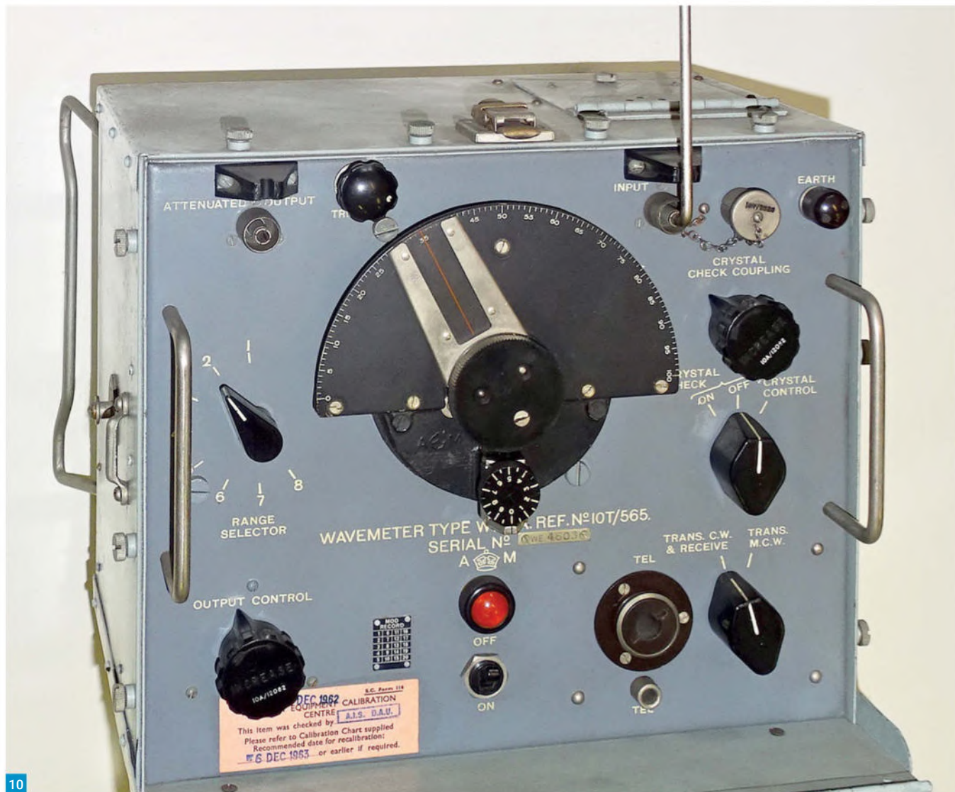
Fig. 10: The W1191A heterodyne wavemeter covers 100kHz to 20MHz in eight ranges.
