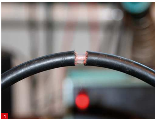
Fig. 1: TinySA Ultra on 3D Printed Stand. Fig. 2: Shielded Loop, which can provide a 30dB null. Fig. 3: Cheap PL259s are good enough in this application. Fig. 4: One end of the cable does not connect to the inner of the PL259. Fig. 5: Cut in the outer braid of the coax cable at the apex of the loop. Fig. 6: Map depicting DF
