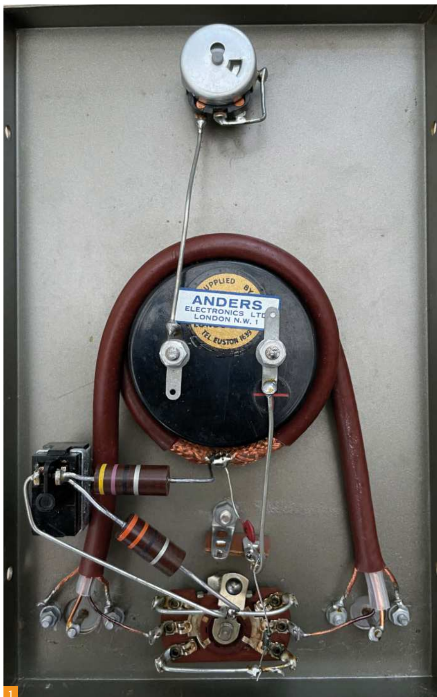
Fig. 1: Inside a classic VSWR meter circa 1960s. Fig. 2: Original KW VSWR meter 75/50Ω, C2V Digital VSWR Power meter, Bird 43 with PEP board. Fig. 3: C2V front panel – switched on. Fig. 4: Inside the C2V software-controlled meter ferrite toroid sensing.
