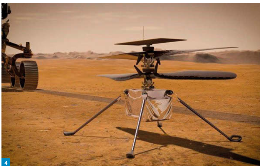
Fig. 4: The highly successful Mars helicopter 'Ingenuity' operating near 2.3GHz on its 45th flight as I type. How fantastic is that reality! However, if it lands below the mobile base, it is simply lost apart from unpredictable terrain dependent diffraction scatter. On Mars that is easy to do because of the weak beam bending due to the sparse atmosphere compared to the Earth, as illustrated in figure (1) if you imagine the slope as nearly vertical. It is vertical on most of the moon (however it does have polar ice so some vapour there). So, microwave propagation understanding including diffraction is critically important.
