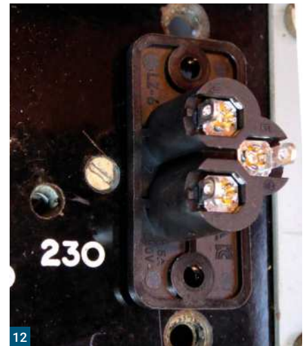
Fig. 6: The two Eddystone 840As. Fig. 7: Non-polarised power inlet on the 840A. Figs 8 & 9: The two different power switch connections. Fig. 10: Rubber power connector. Fig. 11: IEC C6 connector fitted. Fig. 12: IEC connector offered up to rear panel.
