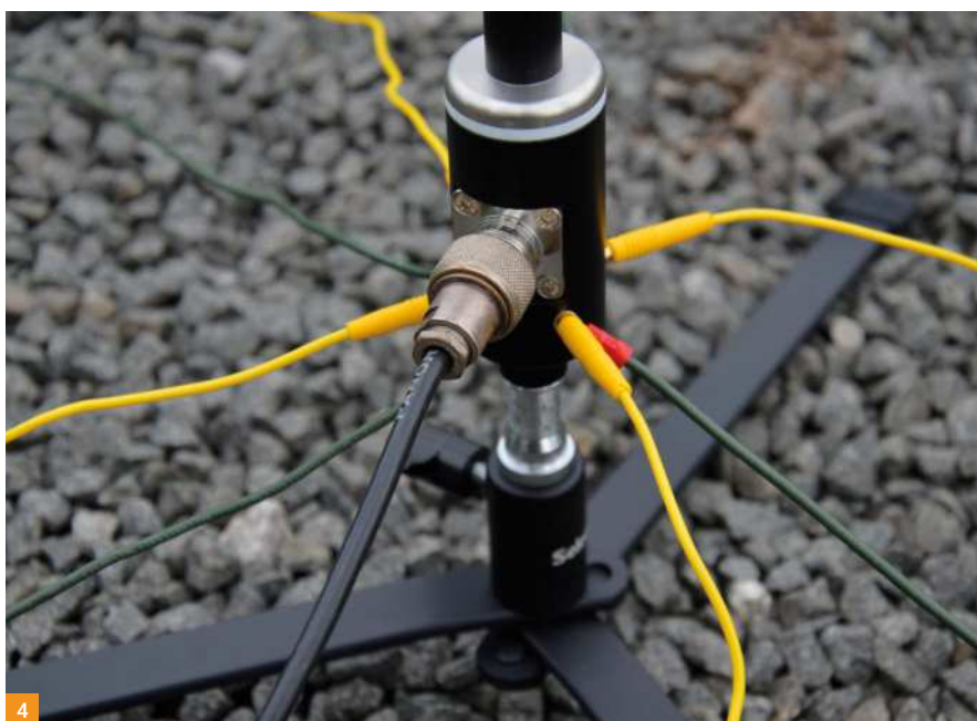
Fig. 4: Antenna base with additional radials, on hard standing.
