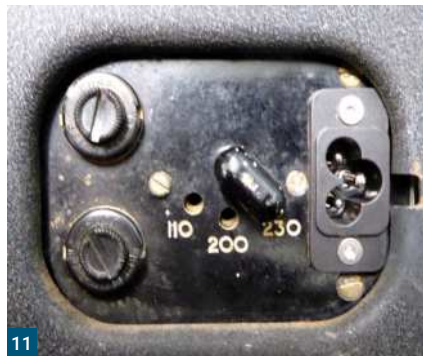
Fig. 6: The two Eddystone 840As. Fig. 7: Non-polarised power inlet on the 840A. Figs 8 & 9: The two different power switch connections. Fig. 10: Rubber power connector. Fig. 11: IEC C6 connector fitted. Fig. 12: IEC connector offered up to rear panel.
