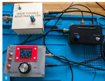
Photo 1: Little Roo parts. Photo 2: The completed Little Roo for the CW end of 40m. Photo 3: Completed and boxed Little Roo. Photo 4: Super Sudden parts. Photo 5: Super Sudden PCB, topside. Photo 6: Super Sudden PCB, copper side. Photo 7: Completed Super Sudden PCB. Photo 8: The Arduino VFO, adjustable BPF and Super Sudden receiver. Photo 9: The boxed Super Sudden (right) with boxed VFO and BPF. Photo 10: QRP Labs receiver and polyphase kits. Photo 11: The completed receiver and polyphase modules. Photo 12: The receiver 'lash up'. Photo 13: The BP-1a BPF kit. Photo 14: The completed BP-1a. Photo 15: The completed and boxed BP-1a.
