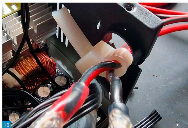
Fig. 8: Connect the green (power on) wire to one of the DC ground wires. Fig. 9: Heatshrink the final pair of wires after soldering. Fig. 10: Use a heavy-duty cable tie to secure the main DC power leads. Fig. 11: And resecure the top cover.
