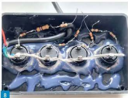
Fig. 1: The parts needed for the project. Fig. 2: Marking the switch positions. Fig. 3: Switch and cable holes drilled. Fig. 4: Switches mounted with connection tabs aligned. Fig. 5: The basic wiring arrangement. Fig. 6: Resistors soldered together for the correct value. Fig. 7: The ground wire connected. Fig. 8: Connecting the resistors. Fig. 9: Ready to go. Fig. 10: Connections to the plug. Fig. 11: The completed keypad.
