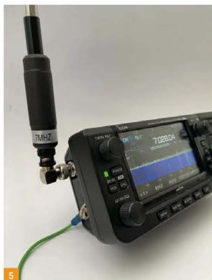
Photo 1: The antenna and loading coils. Photo 2: using a mag mount with the FT-818nd. Photo 3: Attached to a gutter mount – an easy swap between VHF and HF. Photo 4: Using the KX3 on 21MHz. Photo 5: Using the IC-705 on 7MHz, suitably earthed. Photo 6: 28MHz and -MHz inductors.
