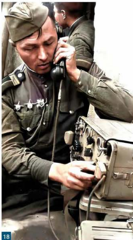
Fig. 13: Portable wireless 3P (Western descriptor 3R) replaced the older RB set for communication down to battalion level. Batteries supplied the power receiving, but for transmitting a hand-cranked generator was required. Fig. 14: This 3P (3R) radio is sitting on its battery case and could be set up in under three minutes. It had a range of up to 15 miles when using voice mode Fig. 15: Over 800,000 women served in front line roles in the Red Army during the war. This Signaller is receiving a message on the 3P (3R) wireless. Note the carrying straps used when transporting the set as a backpack. Fig. 16: The 1940s 6PK man-pack wireless, the forerunner of the RB-M, is popular with radio amateurs, but has become scarce. As a price guide, the popular 1970s USSR P407 (R407) man-pack radio sells on eBay for £600-£700. Fig. 17: The short-wave RB-M radio at battalion level and above. Extremely portable at only 13.5kg it had a range of six miles on the AM band for voice, but as a ground station, using a 7m mast, the range was 18 miles for voice and 50 miles for CW. (radioscanner.ru) Fig. 18: A Soviet Starshina (Sergeant Major) operates a RB-M radio during the battle of Berlin, April 1945.
