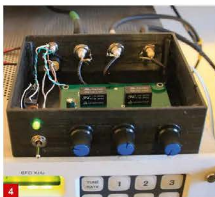
Fig. 1: Circuit taken from the eBay page. Fig. 2: Completed board topside. Fig. 3: Completed board underside. Fig. 4: Assembled eliminator in box. Fig. 5: Assembled and awaiting labels. Fig. 6: Adventist World Radio 15710kHz suffering noise on the left and eliminated to the right. Fig. 7: VDSL QRM top, eliminated at bottom with around 1 S-Point wanted signal loss.
