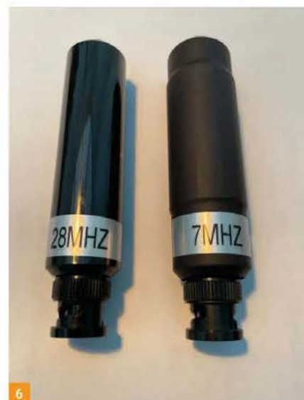
Photo 1: The antenna and loading coils. Photo 2: using a mag mount with the FT-818nd. Photo 3: Attached to a gutter mount – an easy swap between VHF and HF. Photo 4: Using the KX3 on 21MHz. Photo 5: Using the IC-705 on 7MHz, suitably earthed. Photo 6: 28MHz and -MHz inductors.
