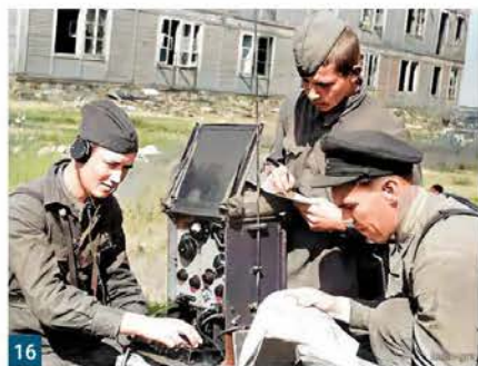
Fig. 13: Portable wireless 3P (Western descriptor 3R) replaced the older RB set for communication down to battalion level. Batteries supplied the power receiving, but for transmitting a hand-cranked generator was required. Fig. 14: This 3P (3R) radio is sitting on its battery case and could be set up in under three minutes. It had a range of up to 15 miles when using voice mode Fig. 15: Over 800,000 women served in front line roles in the Red Army during the war. This Signaller is receiving a message on the 3P (3R) wireless. Note the carrying straps used when transporting the set as a backpack. Fig. 16: The 1940s 6PK man-pack wireless, the forerunner of the RB-M, is popular with radio amateurs, but has become scarce. As a price guide, the popular 1970s USSR P407 (R407) man-pack radio sells on eBay for £600-£700. Fig. 17: The short-wave RB-M radio at battalion level and above. Extremely portable at only 13.5kg it had a range of six miles on the AM band for voice, but as a ground station, using a 7m mast, the range was 18 miles for voice and 50 miles for CW. (radioscanner.ru) Fig. 18: A Soviet Starshina (Sergeant Major) operates a RB-M radio during the battle of Berlin, April 1945.
