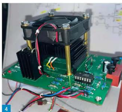
Fig. 1: Advance PMG-24-3 power supply. Fig. 2: 2-wire and 4-wire operation. Fig. 3: Circuit diagram of variable power supply add on. Fig. 4: Assembled PCB with heatsink fan. Fig. 5: Assembly of the fan above the heatsink. Fig. 6: Details of the four pillars.
