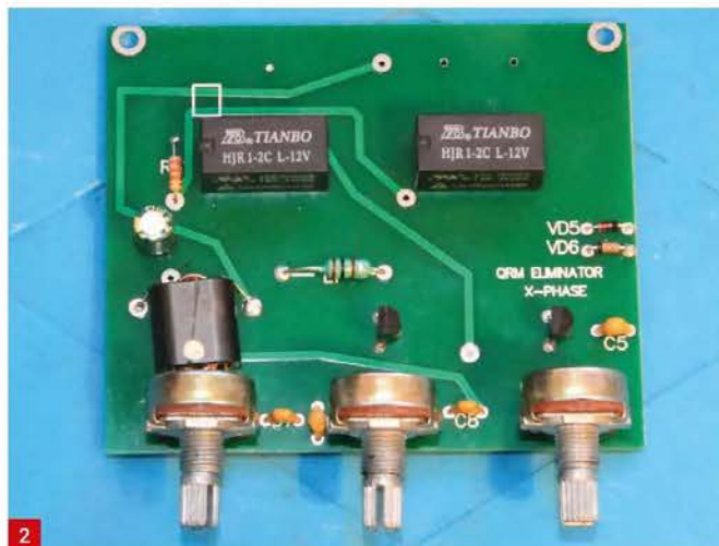
Fig. 1: Circuit taken from the eBay page. Fig. 2: Completed board topside. Fig. 3: Completed board underside. Fig. 4: Assembled eliminator in box. Fig. 5: Assembled and awaiting labels. Fig. 6: Adventist World Radio 15710kHz suffering noise on the left and eliminated to the right. Fig. 7: VDSL QRM top, eliminated at bottom with around 1 S-Point wanted signal loss.
