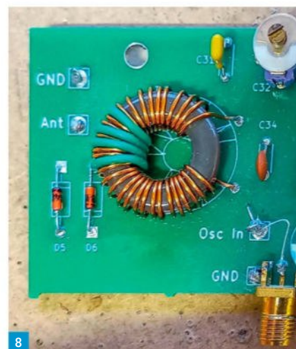
Fig. 6: The audio preamplifier assembled. Fig. 7: The product detector assembled. Fig. 8: The bandpass filter assembled.
