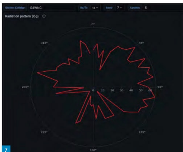
Fig. 7: Radiation pattern plot from the WSPR Live site. Fig. 8: WSPR Live 3-D plot of live activity on 10m.
