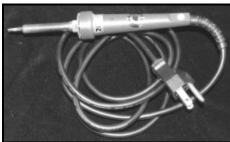
This iron is an inexpensive, adjustable 25-40 watt unit, and quite suitable for constructing this type of kit.
