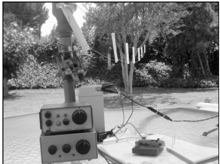
Two transceivers and the NorCal BLT tuner, which was literally hanging from the end of the W3EDP end-fed's parallel feedline, were used for initial testing of the antenna at KI6SN.
