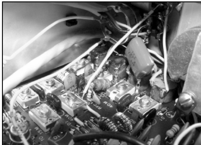
This is a close up of the RFC/parallel RC mod that will reverse bias any non-selected bandswitching diodes (D1-4). This mod is easily reversed. It definitely tames the motorboating on the transmitted signal.
