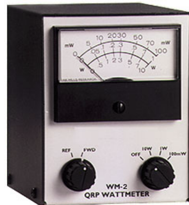
The Oak Hills Research WM-2 was designed specifically for the QRP operator. The unit operates from 300 KHz to 54 MHz. It will measure forward and reflected power at QRP levels down to 5mW. (See www.ohr.com )
