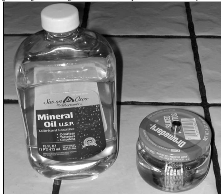
Mineral oil, available off the shelf in the laxative area of your local drug store, is a long-used medium in dummy loads.
