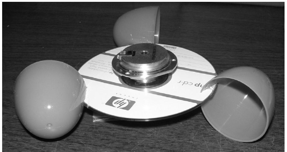
Anemometer with center hub cap removed to show brushless DC motor.
