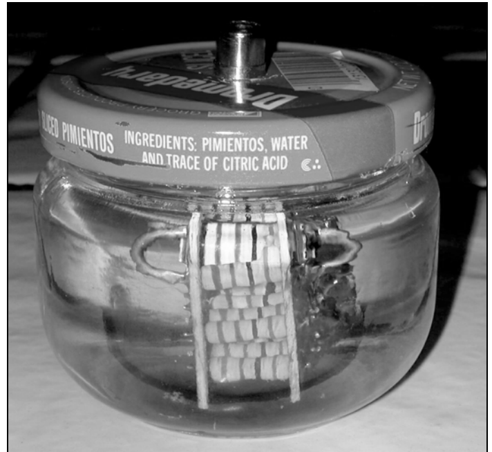
At KI6SN, the resistor load, suspended in mineral oil, is capable of comfortably handling more than 20-watts of key down power.
