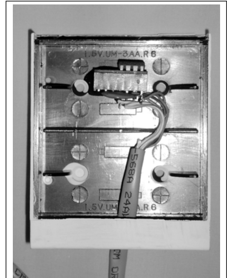
No-hands Clock DS1620 temperature sensor mounted in weather resistant enclosure. Device mounted in IC socket that is epoxied in an ‘AA’ battery case. Outside of case is painted white to avoid heat absorption errors.
