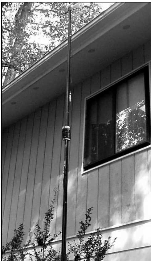
Figure 4: Loading Coil on Pole
