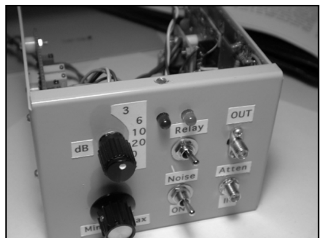
Figure 5: Calibrated noise source project
