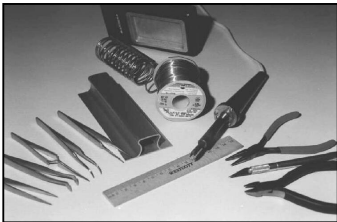
Solder & assembly tools used at K7QO chain nose pliers (a finer tip than needle nose pliers), Exacto hobby knife with #11 blade, and Sears diagonal cutters (4.5" Craftsman #45171).
