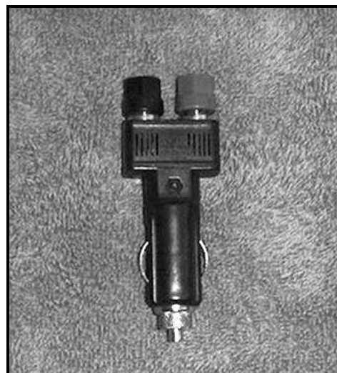
Photo 1: Radio Shack Lighter Plug with Binding Post Connections
