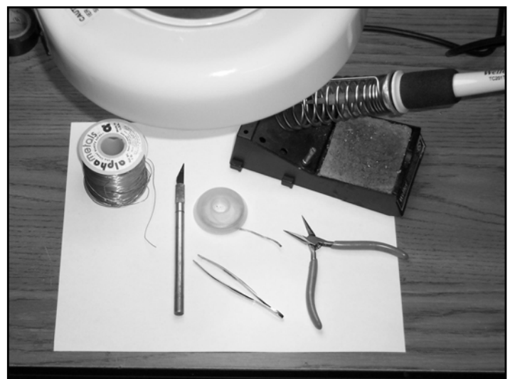
Figure 2: SMT soldering tools: magnifying lamp, .015" solder, fine-tipped soldering iron, tweezers, Xacto knife, Solder-Wick, needle-nose pliers.
