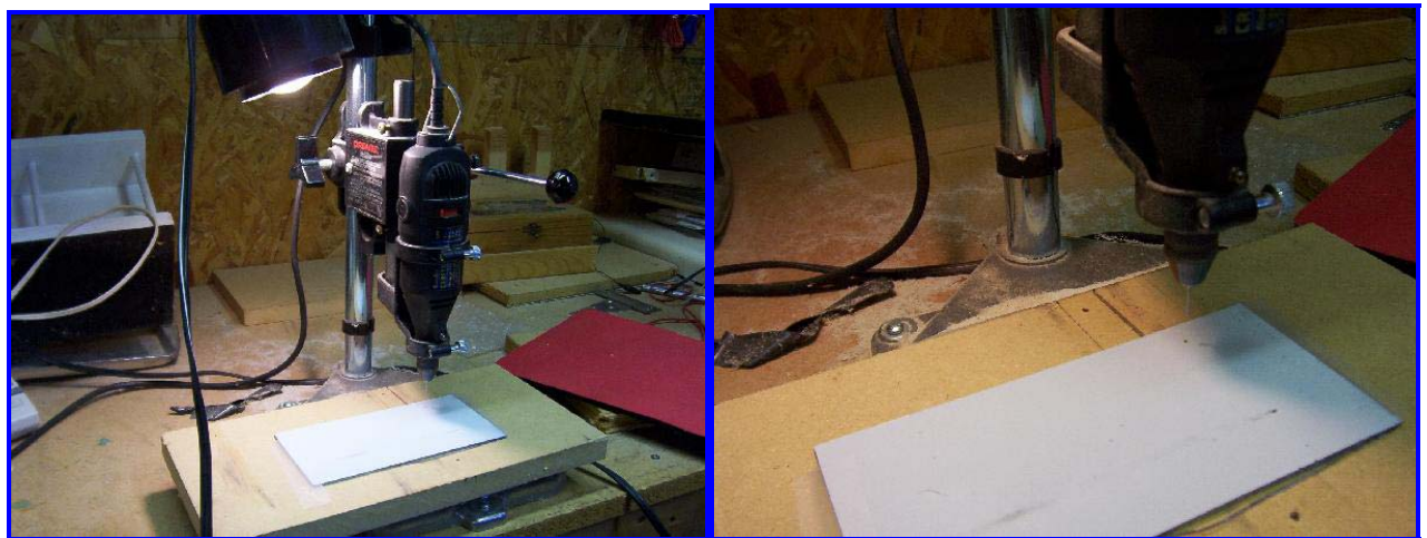
Here is Bill's Dremel Drill Press for drilling holes after the PCB has been etched.
