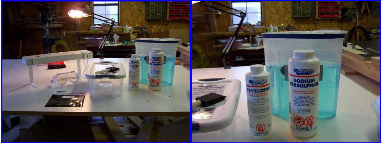
Here we are able to see the exposure kit, developer tank, a pre-sensitized board (in the black plastic bag) foam brush and SAFETY GLASSES "WEAR THEM"
