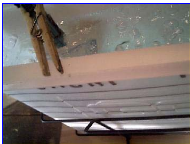
After exposure and the developer bath, even though the pictures are dark you can see the traces
