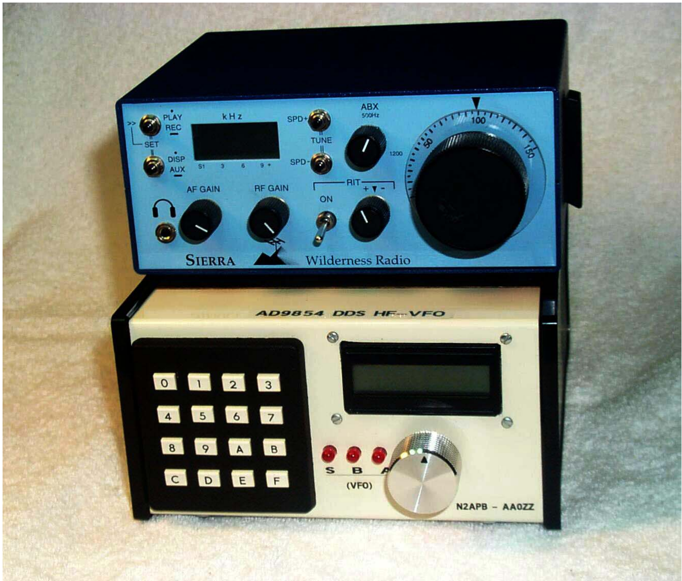
Here's the front view of the stacked pair: the Wilderness Radio Sierra QRP transceiver (top) and the AA0ZZ 9850 High Performance HF VFO (bottom). During operation, frequency tuning is done (and displayed) on the external HF VFO, while the dial and display on the Sierra is not used.
