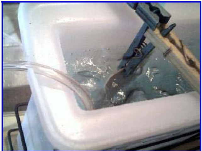
After exposure and the developer bath, even though the pictures are dark you can see the traces
