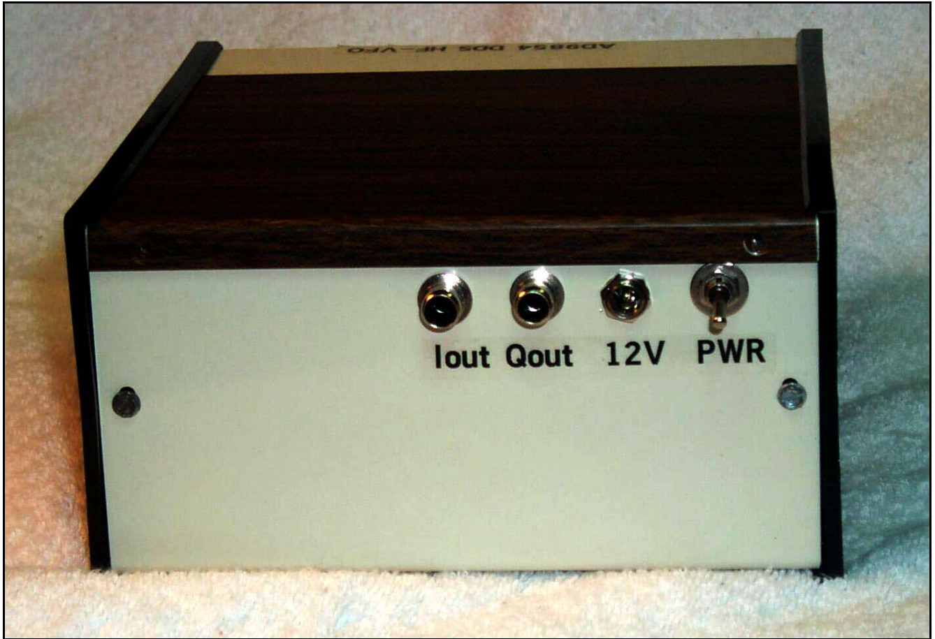
The rear panel provides connections for the two quadrature output signals (I and Q), the power jack and the power switch.
