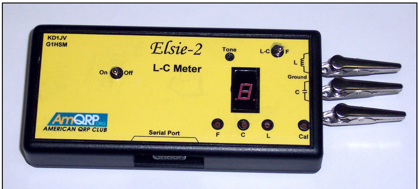
Completed prototype of the Elsie-PCB project, nicely enclosed in the Hammond 1595 plastic case.
