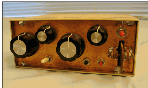
Front panel of rig, with controls as follows: Top Row = VFO1, Fine Tune, VFO2, RF Gain, Power Bottom Row = VFO Switch, FreqMite Button (black), Keyer Button (red), Keyer Paddle Control. Labels are on front edge of top panel.
