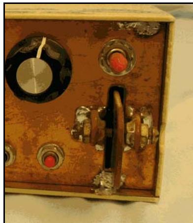
Finished Single Paddle Installation
