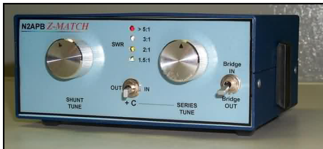
Classic Z-Match in an N2APB-enclosure, combined with the Rainbow Tuner SWR Bridge (LEDs on front panel)
