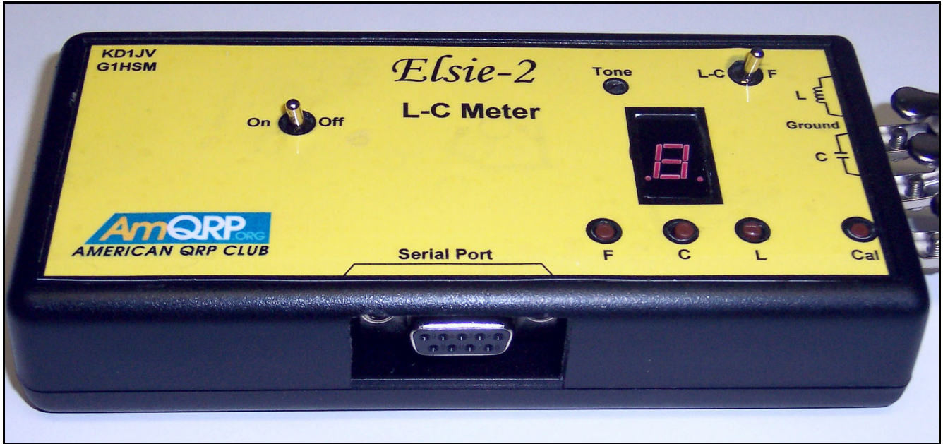
Side view of the Elsie-PCB enclosure, showing the connector for serial connection to the PC (primarily used for data collection during use.)
