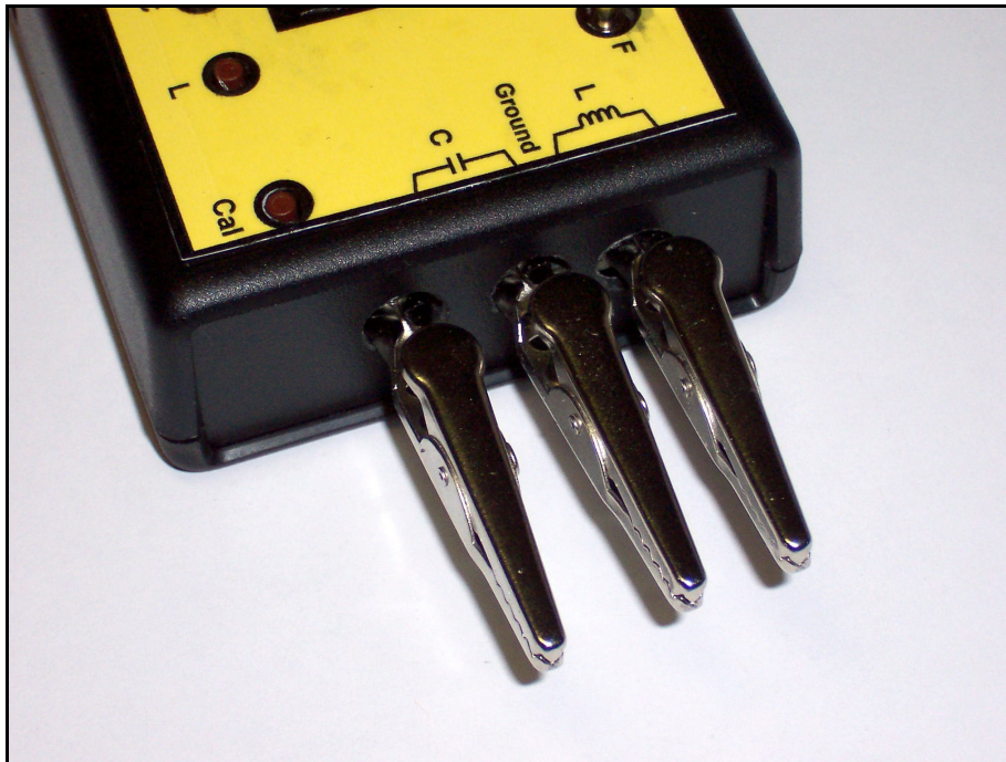
End view of the Elsie-PCB enclosure, showing how the alligator clips protrude through the end panel to allow easy clip-on of the inductor or capacitor under test.
