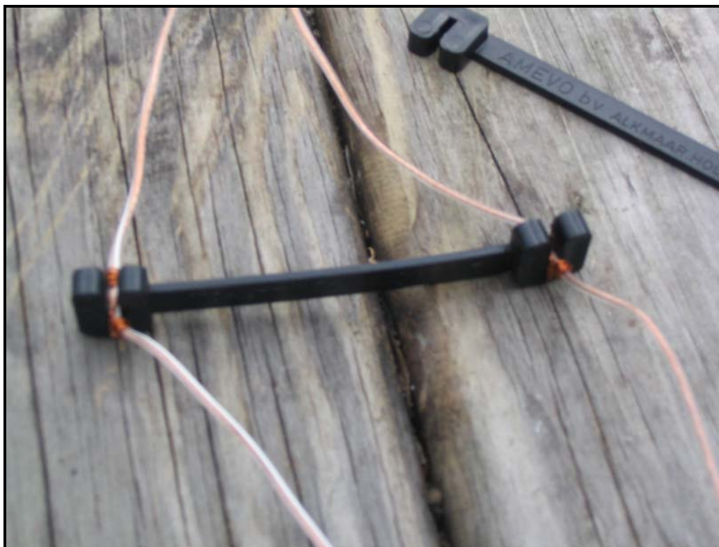
Legs of W3EDP held apart by lightweight spacers.
