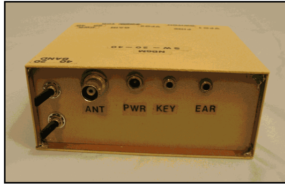
Rear of rig, showing band switches to the left, and the connectors shared by the two boards
