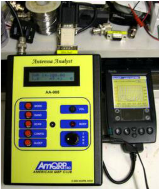
Mike WA6FXT snapped a couple of nice photos of the connection to his Palm IIIc with the simpler connector arrangement using a null modem adapter (short white adapter) along with a 9-pin gender changer (shorter yellow adapter).
