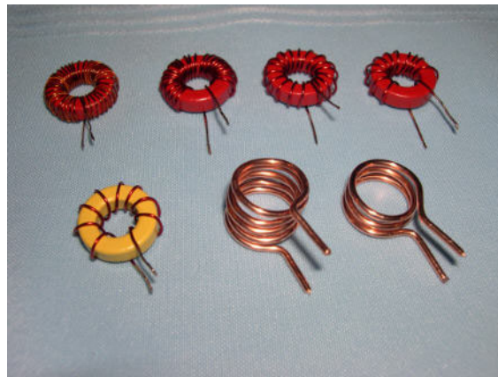
TOROIDS AND COILS COMPLETED
