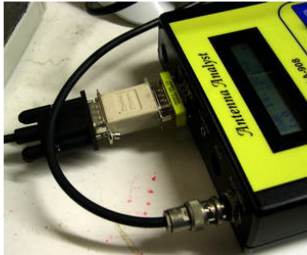
Mike WA6FXT snapped a couple of nice photos of the connection to his Palm IIIc with the simpler connector arrangement using a null modem adapter (short white adapter) along with a 9-pin gender changer (shorter yellow adapter).
