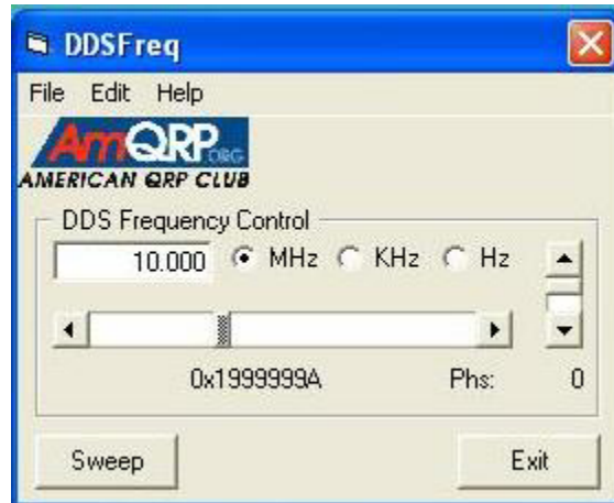
The first window to appear when running DDSFreq provides control of the control word sent to the DDS chip.
