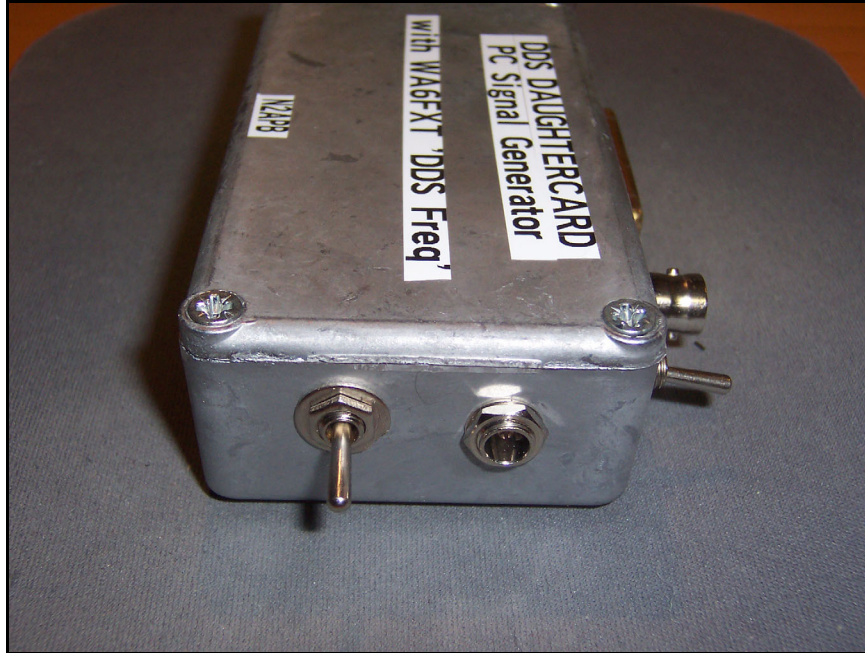
End view of the enclosure shows the +V power jack and switch.
