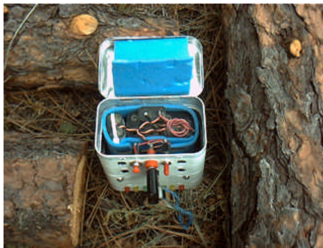
Battery pack wrapped in closed-cell foam
