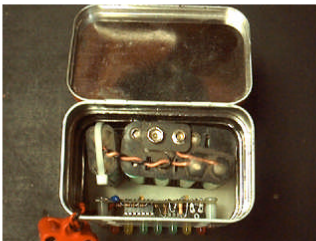
Checking battery pack fit.
