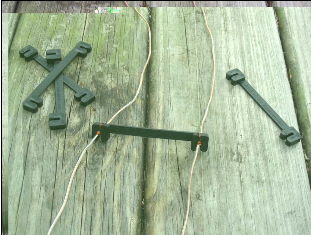
Spacers at work on two legs of W3EDP end-fed antenna
