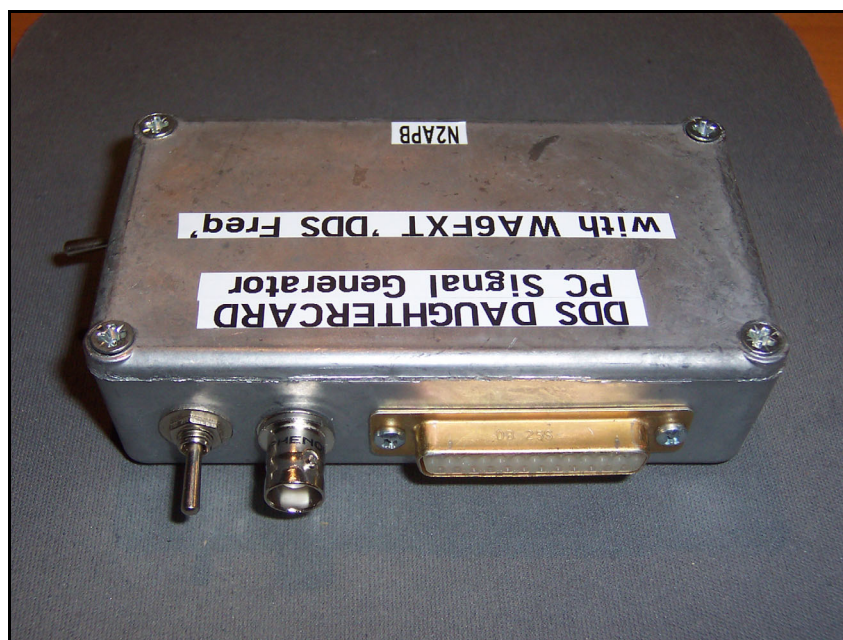
Side view of the enclosure shows the connectors for the parallel port cable (right), BNC for the RF output (middle), and the toggle switch (left) to switch in/out the 50-ohm load resistor when needed.
