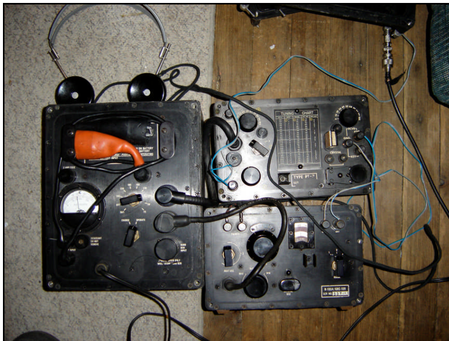
Here is the entire GRC-109 Special Forces/CIA spy radio station set up for operation. This station is a gas to use, despite the wide IF bandwidth on the R-1004 receiver. I have tried a passive AF filter on this radio with limited success. The transmitter has a nice little "chirp" that makes it stand out in a crowd.
