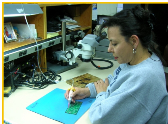
Fig. 21 – Professional assembler Mary Ellen Chavez applies solder paste to a PCB preparatory to reflow soldering.
