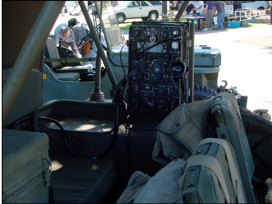
Here is an old GRC-9 mounted in a flat fendered jeep from the post WWII era. The GRC-9 saw action in Korea, Viet Nam and around the world. It is still in some National Guard Units commo bunkers!
