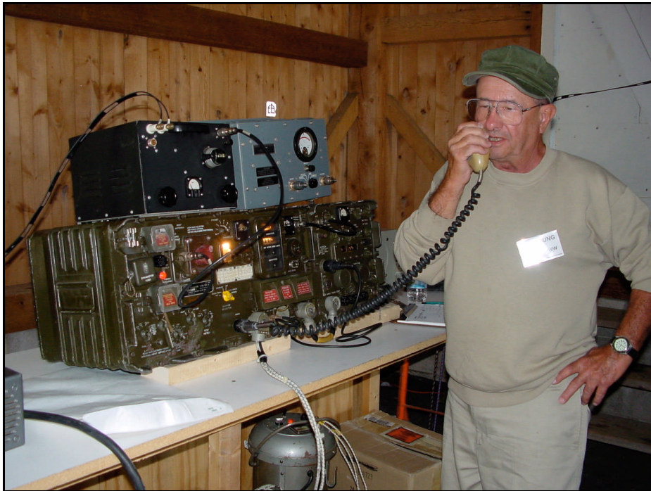
These photos show Ted Young, W3PWW operating his AN/GRC-19 HF radio set. This unit is made up of the T-195 HF transmitter (with a really wild electro-mechanical automatic antenna tuner built in!) and the R-392 receiver (which is a mobile version of the Collins R-390 fixed station receiver). This unit is capable of several hundred watts output and can transmit CW/AM and SSB. It's big, it's noisy, and it has motors!!!!
