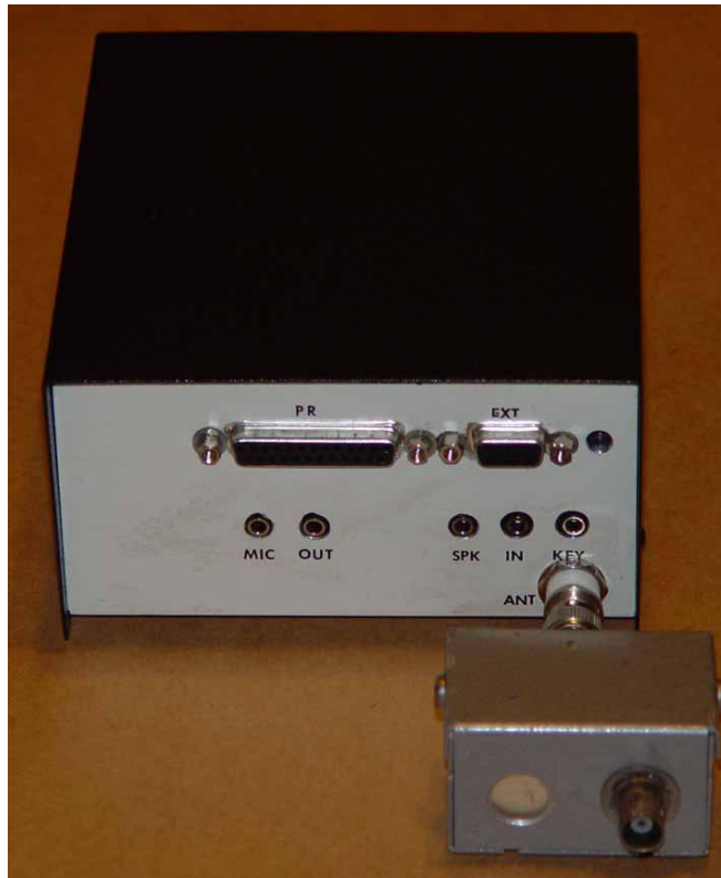
Figure 6 shows an external 20 meter filter used to keep harmonics at -80 dbc when using the 20 watt power amplifier on 20 meters. A relay and band filter board is under construction, which will provide harmonic filtering for all transmit bands used with the 20 watt power amplifier. The SDR-1000 provides a connector to switch the relays needed for changing the filters for the added power amplifier.
