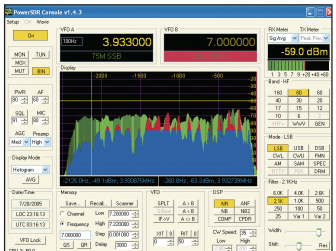
Figure 9—The “histogram” display on 75 meters. Setting the buffers at too low a value while using this display can chop “holes” in the received signal. This is an apparent computer processing issue.
