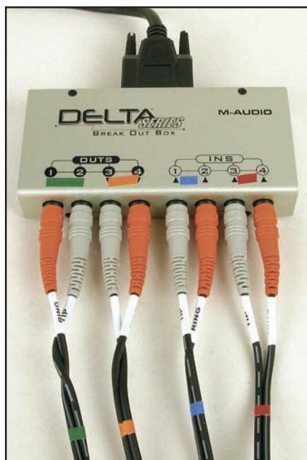
Figure 1—The break-out box for the optional M-Audio Delta 44 professional sound card allows making the connections without crawling behind the PC.
