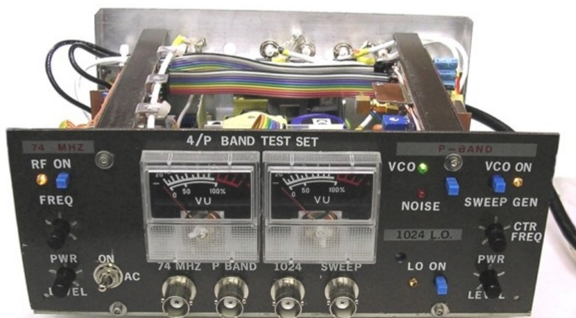
Fig. 23 – A Manhattan-built Test Set used to simulate three VHF receivers and contains a 1024 MHz Local Oscillator
