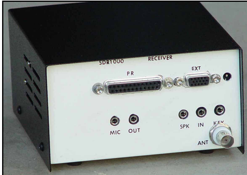
Figure 11: WD6CSV's SDR-1000 mounted in Jameco enclosure with transceiver connectors accessible on the rear panel. Others have used an empty K2 chassis.
