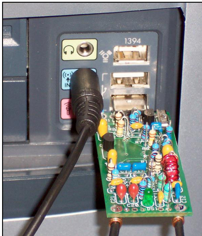
Fig 2: SoftRock-40 pcb plugged into USB port on a desktop computer. The little receiver is powered from the USB port. A cable supplies audio to the 'line in' connector for the PowerSDR software to process the I & Q signals, while another connects to a 40-meter antenna.
