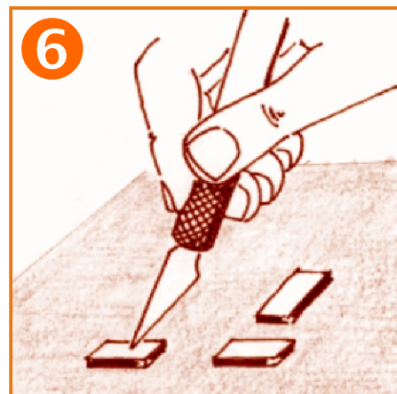
Place the pads onto the drop of glue and position with an Exacto knife, other sharp object or tweezers..
