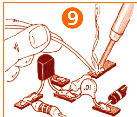
The glued pads become the mounting platforms for the components, soldered in place.
