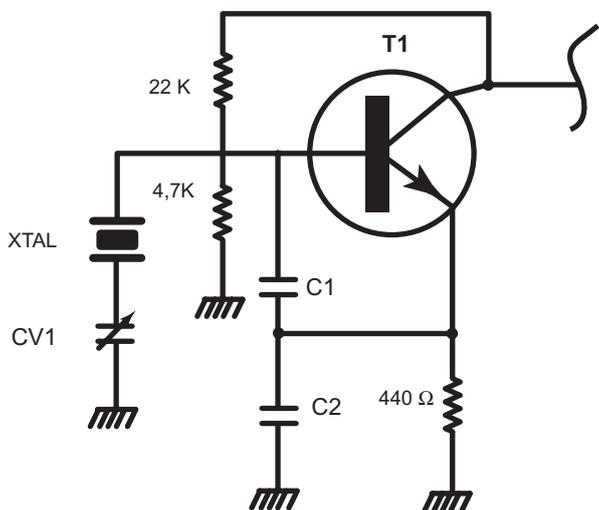
**Figure 2** SCHEMA RESONANCE PARALLELE
