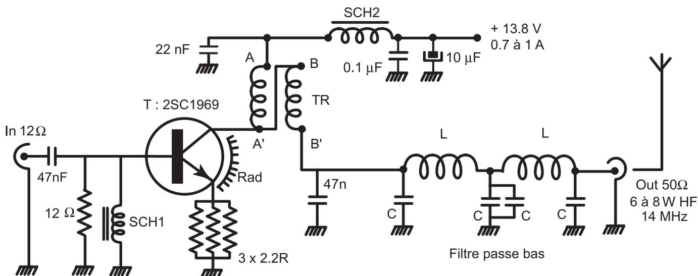
**Figure 3** PA version 6-8 Watts 14 MHz
