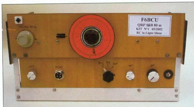
▶ TRANSCIVER QRP/SSB BANDE 80 METRES 2.5 WATTS HF
