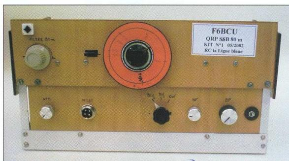
TRANSCIVEUR QRP/SSB BANDE 80 METRES 2.5 WATTS HF
