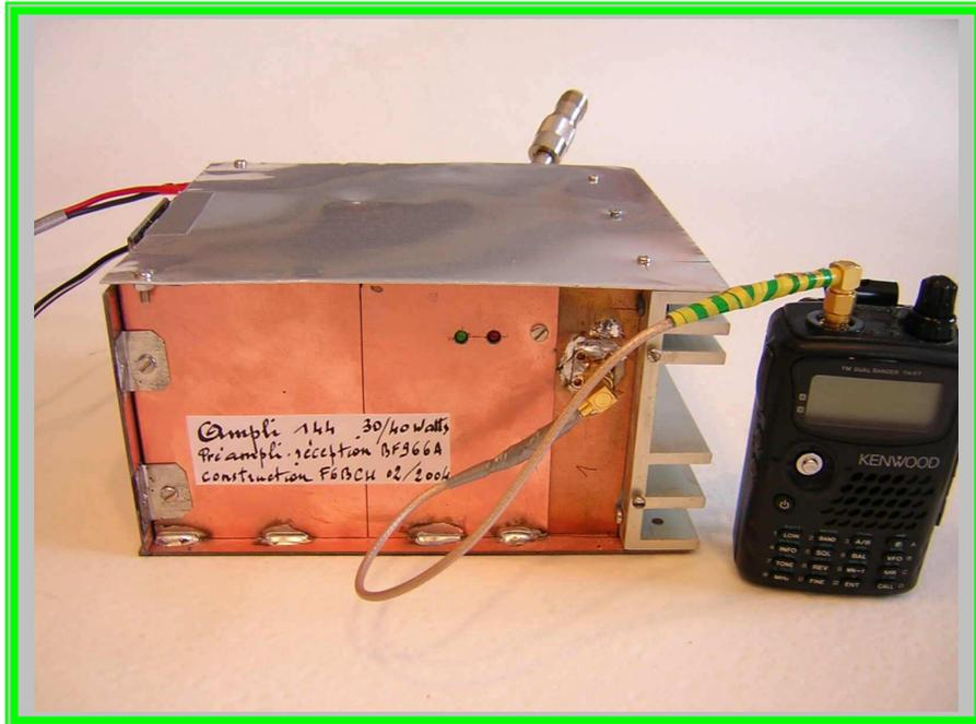
**AMPLIFICATEUR 144/146 FM MOBILE OU PORTABLE GAIN
