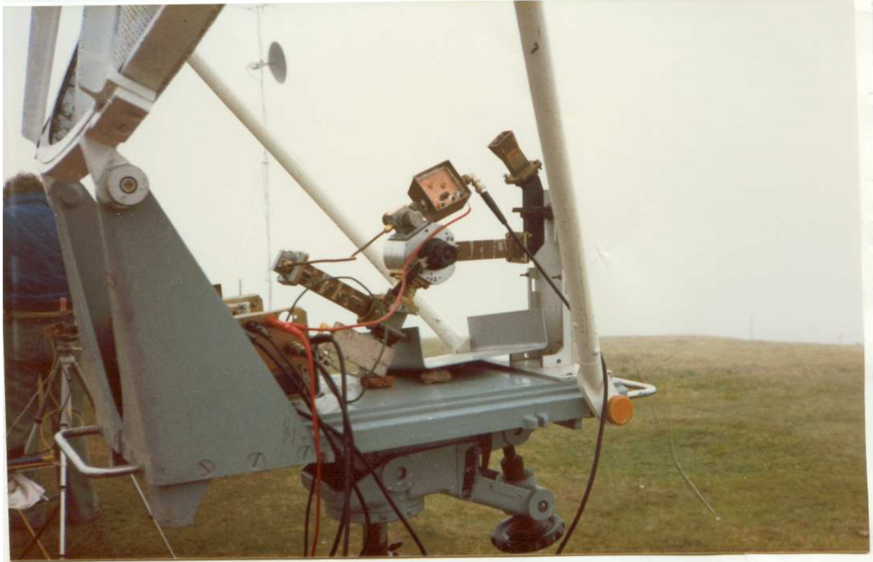
DETAIL Tx 10GHz 7mW HF F6DPM
