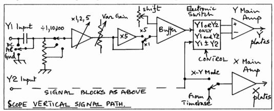
with the spot moving up and down at a speed depending on the applied frequency. The height of the vertical line or band representing the peak to peak voltage.
