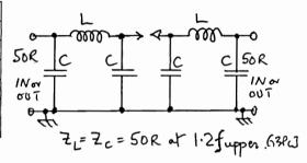
These low pass filters can also be used after a class C amplifier without any internal tuning.
