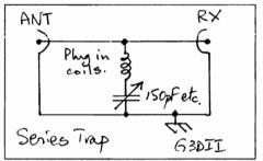
smaller equivalent value parts within the RX case using a trimmer/fixed coil or fixed capacitor/slug tuned coil. Measure the resonant frequency, with a GDO, by shorting out either connector.
