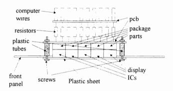
Fig. 2. Upper view of the display attachment
