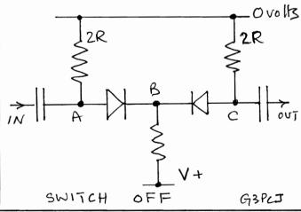
practical circuit, the diodes will have some capacitance so there will be some leakage and the isolation will not be perfect but quite sufficient to protect the receiver's front end filters!
