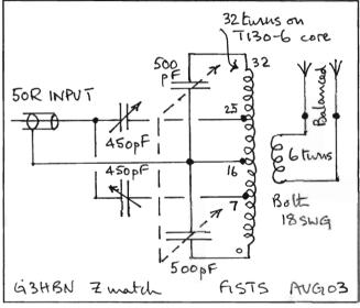
Hene is another AMU but this time using the T match C-L-C approach. It incorporates a RF transformer at the input to the matching section so that the output is (almost) floating and can drive a balanced feed line and antenna. The kit also includes a resistive matching bridge and was reviewed in the July 2003 PW.
