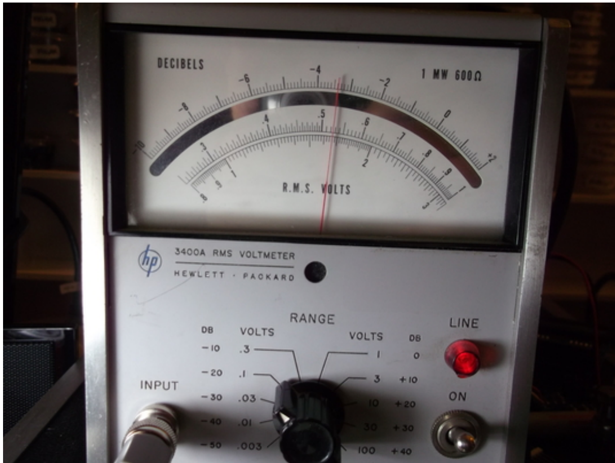
Figure 89: HP3400A RF Voltmeter at 5.1K resistor.
