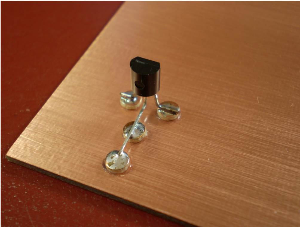
Figure 233: Q1 mounted to pads.
