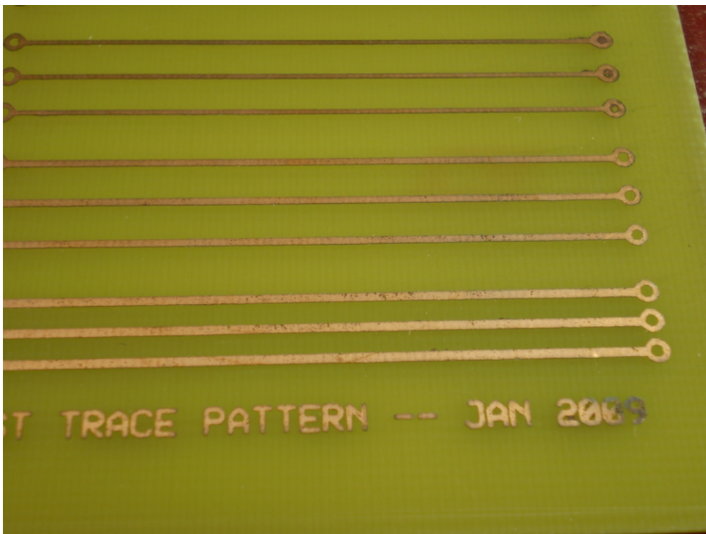
Figure 260: Jan 2009 Test Board after 6 years.
