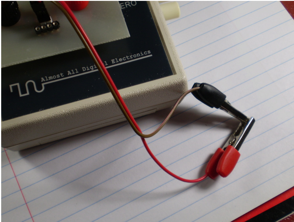
Figure 180: Cables shorted out to calibrate for zero inductance.
