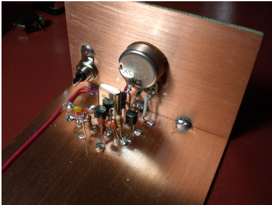
Figure 126: Two Piece fixture to build Manhattan project on.
