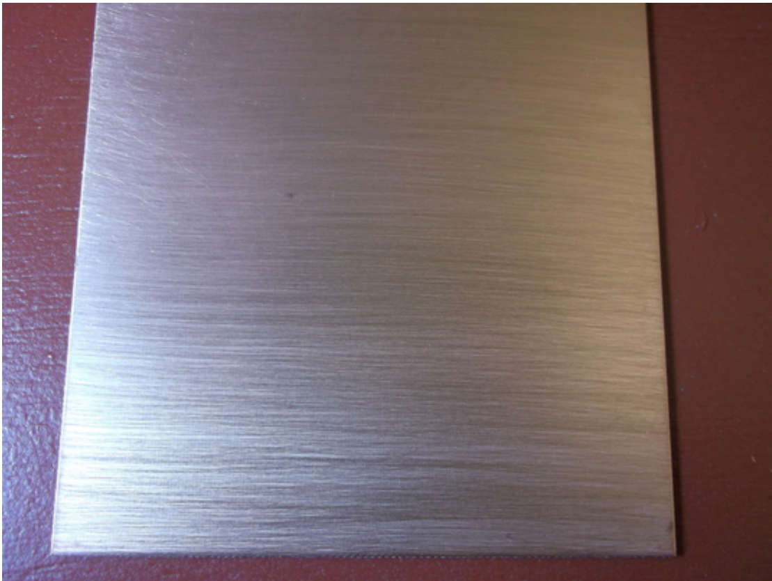
Figure 30: Board Cleaned with 3M Pad.
