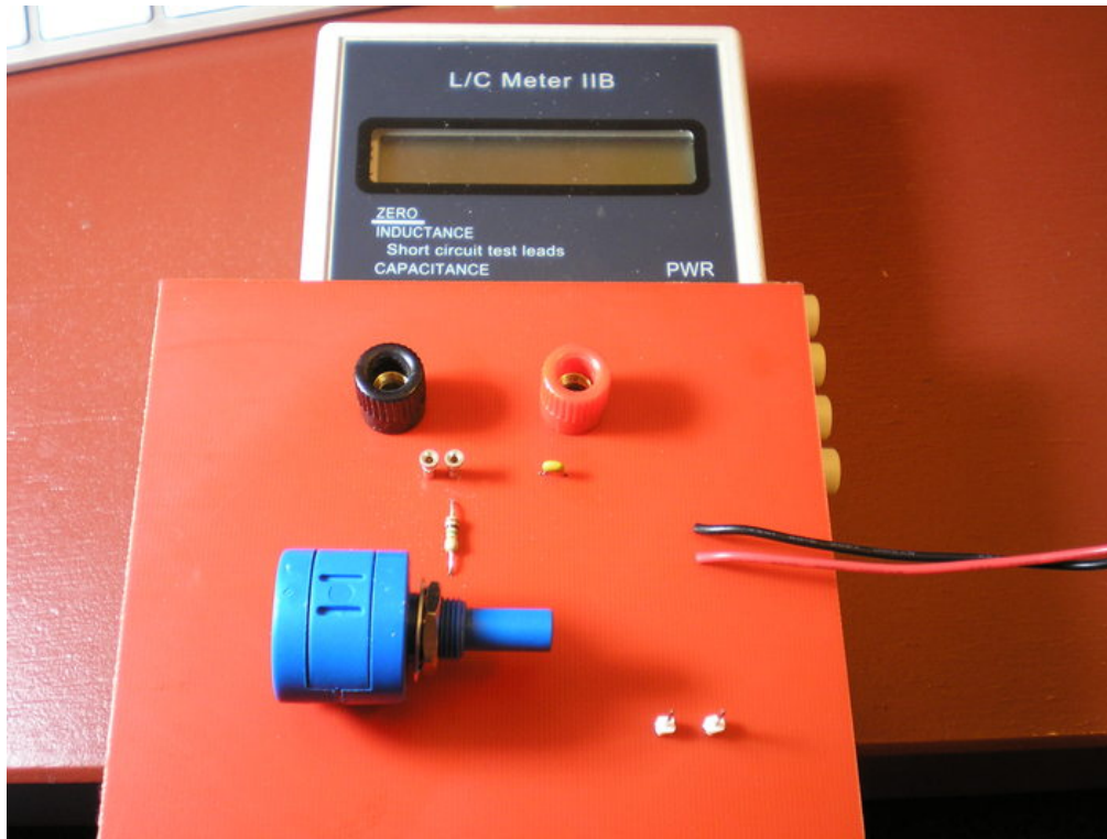
Figure 160: Varactor Fixture attached to AADE L/C Meter
