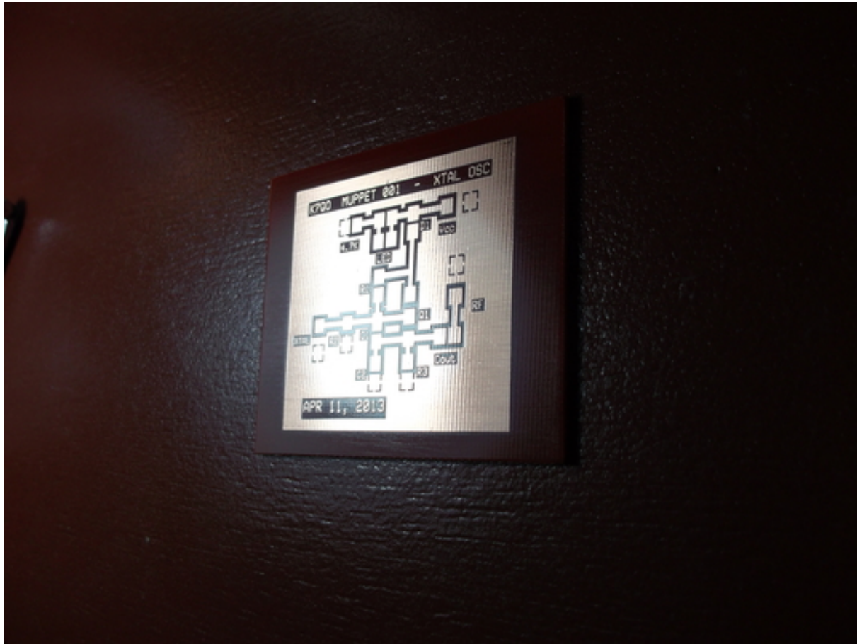
Figure 75: Board coated with light coat of clear Krylon.
