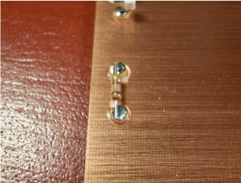
Figure 229: Resistor soldered into place.
