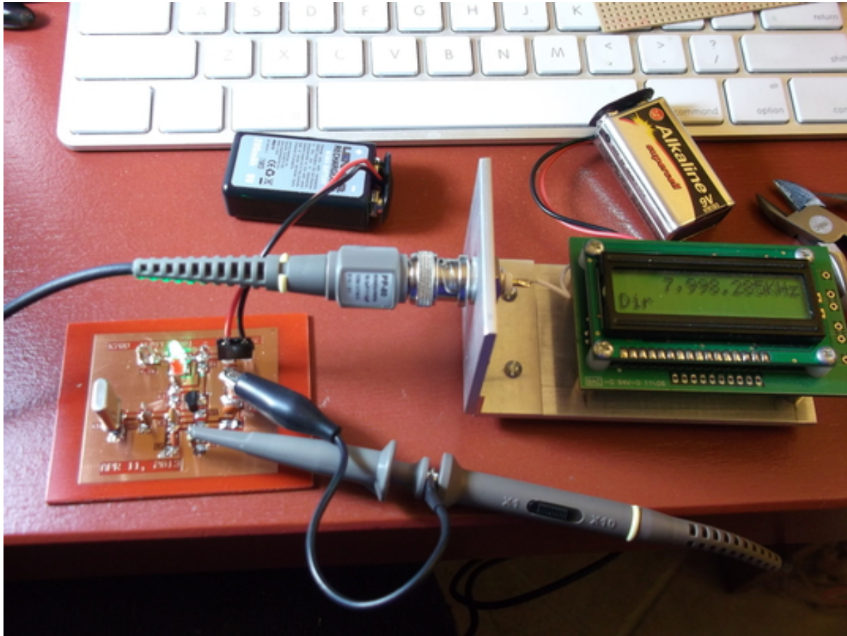
Figure 87: Oscillator up and running and connected to freq counter.
