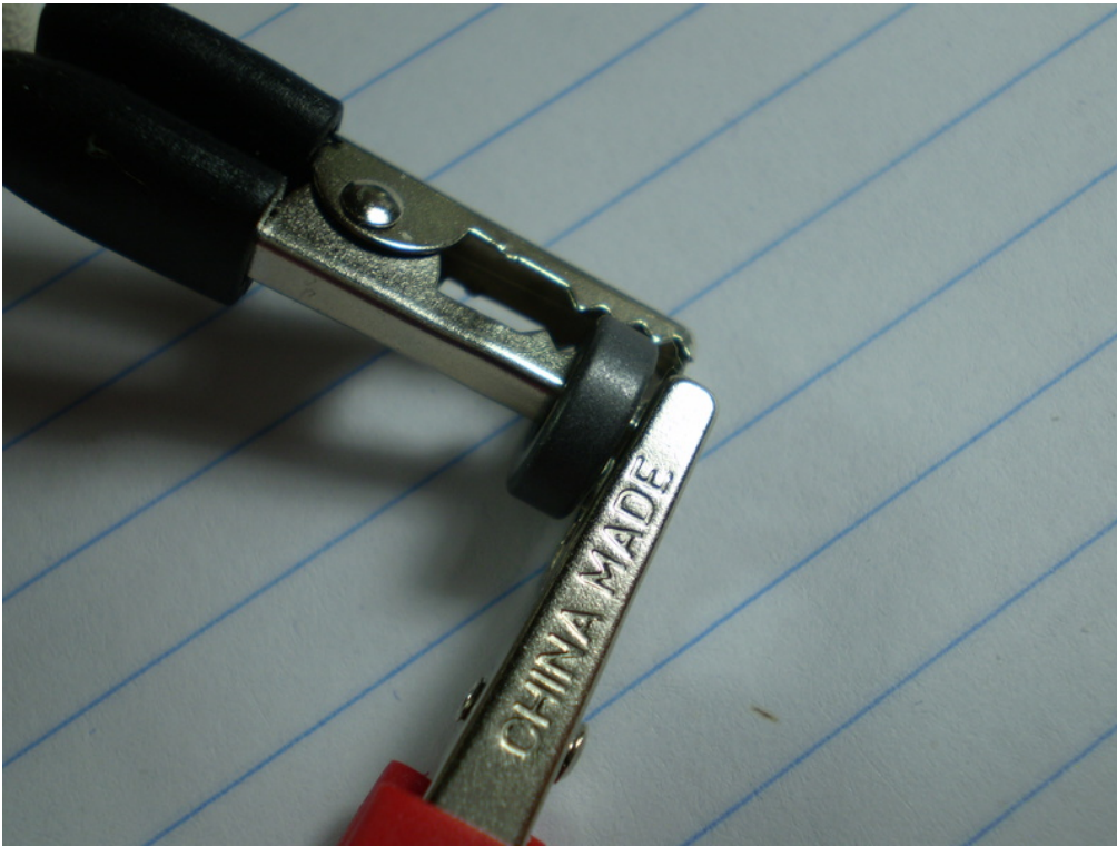
Figure 182: FT37-43 in place.
