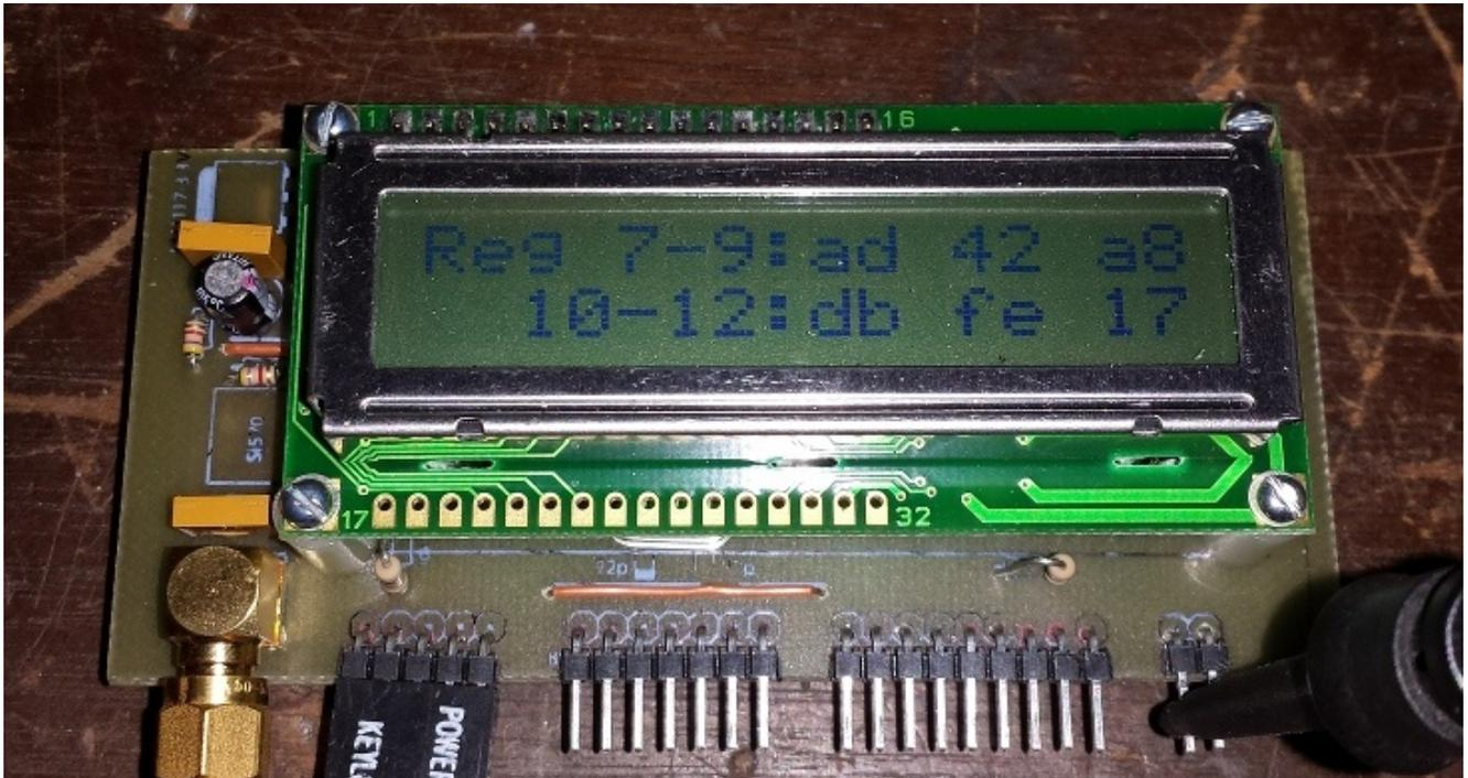
Illustration 18: Display of Si570 register values, as part of the Si570 testing sketch.
