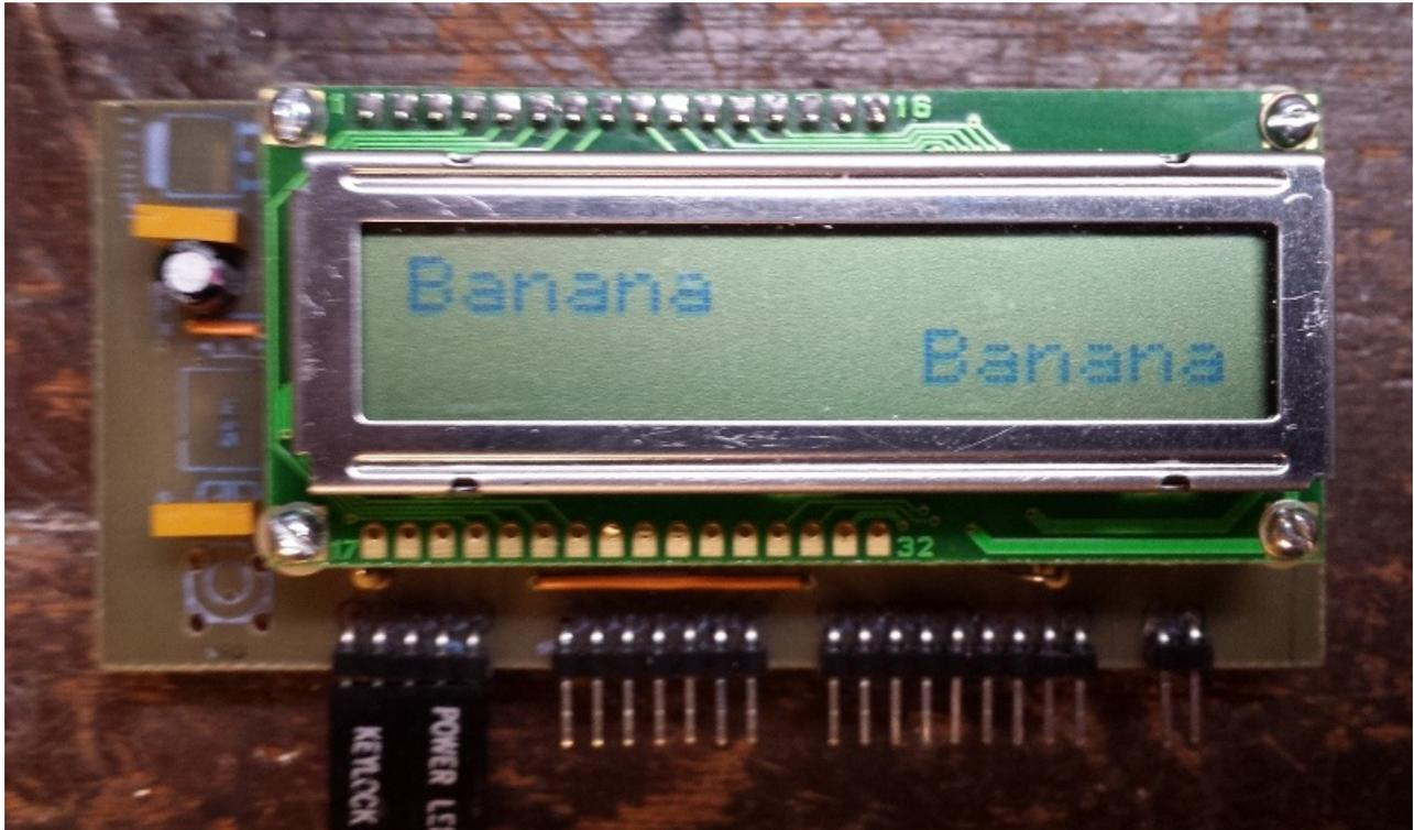
*Illustration 12: LCD display results from the Arduino microcontroller LCD test.*
