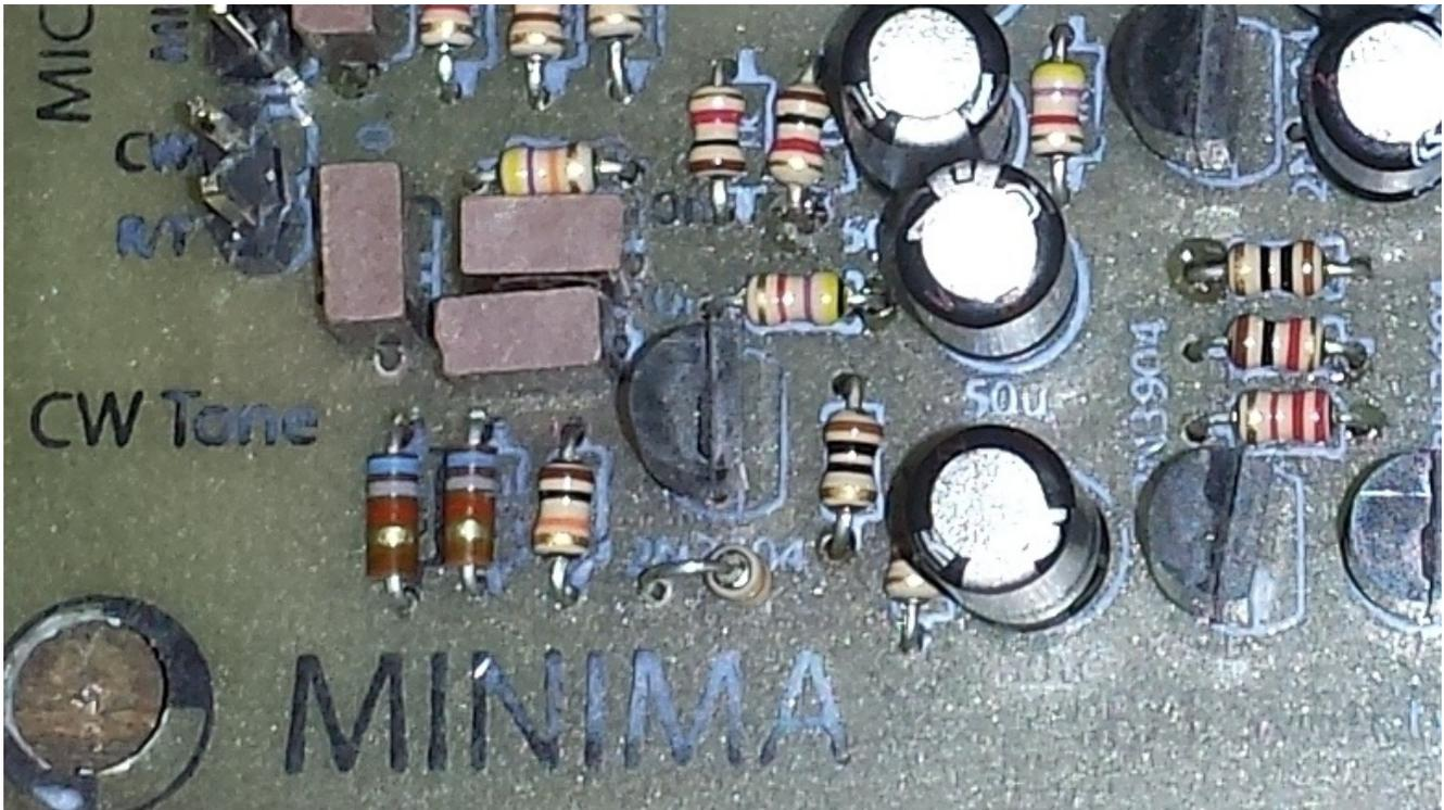
*Illustration 45: Component placement for the Main Board CW Tone Oscillator assembly.*
