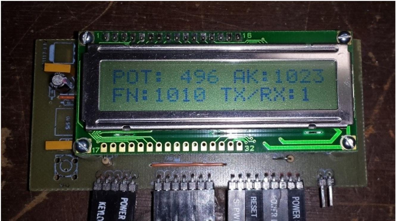
*Illustration 15: Appearance of LCD display for the Arduino Microcontroller I/O Testing sketch.*
