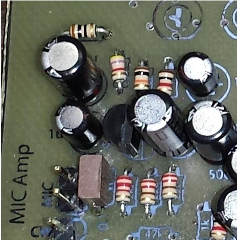
*Illustration 40: Component placement for the Main Board Mic Preamp circuitry.*
