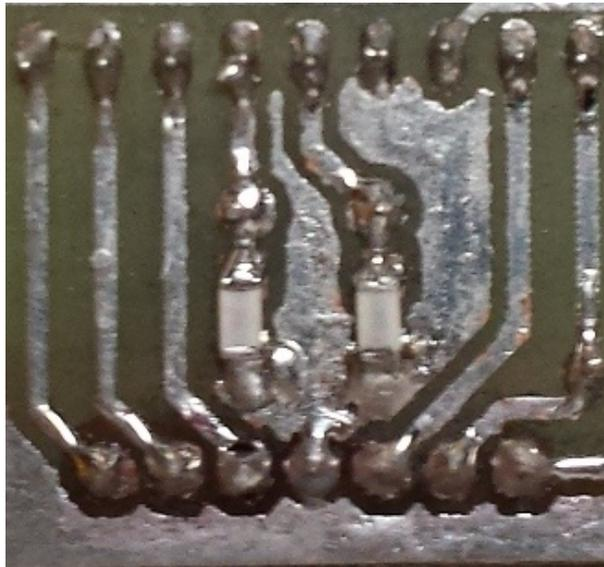
*Illustration 5: Installation of 22 pF capacitors.*
