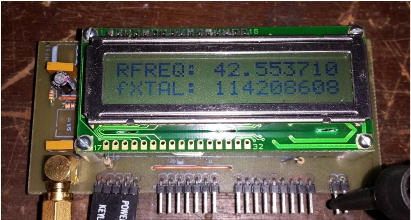
*Illustration 20: Display of the Si570 Reference Frequency (in MHz) and the crystal frequency (in Hz).*
