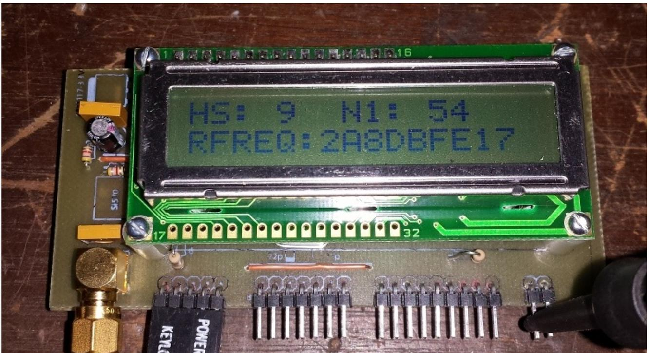
Illustration 19: Display of HS, N1, and RFREQ, as part of the Si570 testing sketch.
