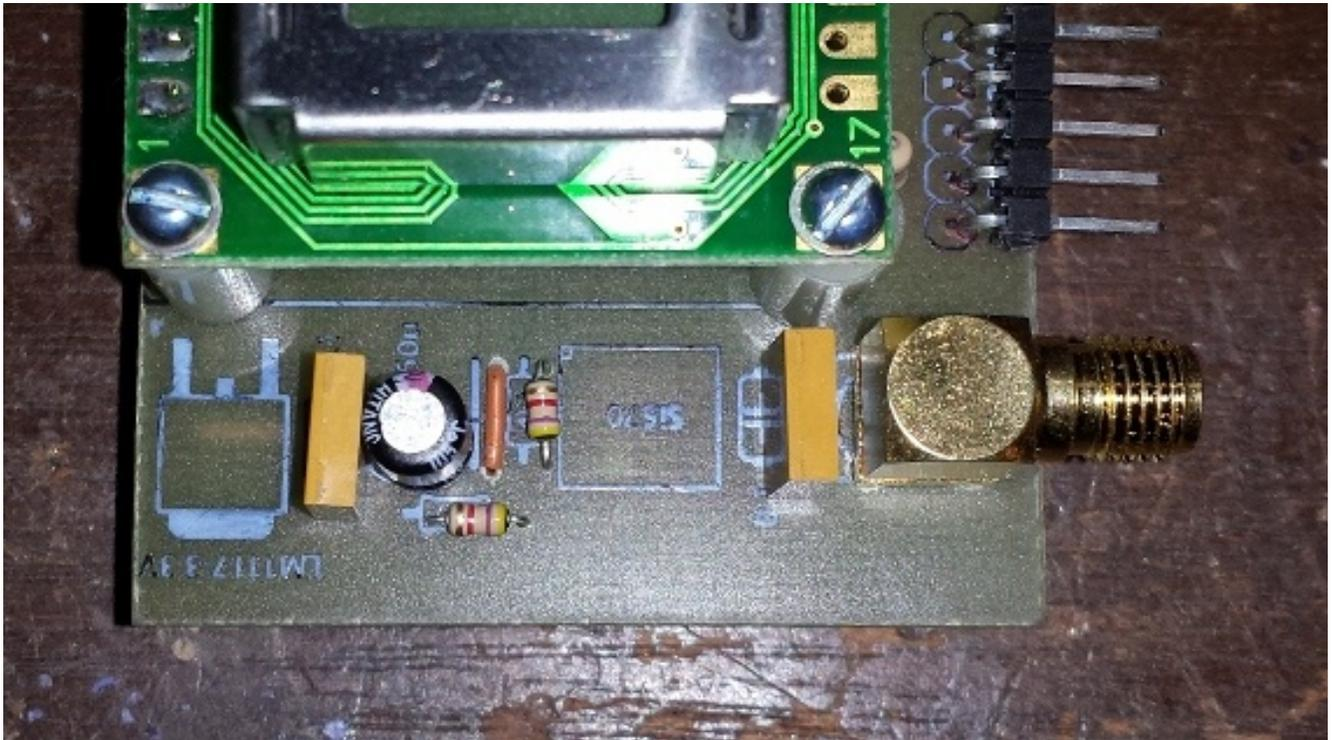
*Illustration 16: Component side of Digital Board with the Si570 support components installed.*
