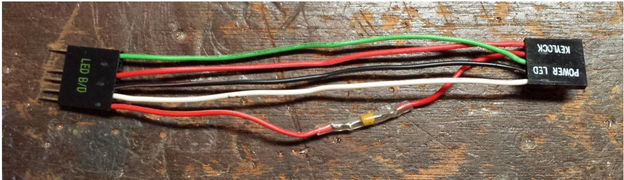
*Illustration 9: Interface cable from the USB-to-TTL serial adapter to the Digital Board.*
