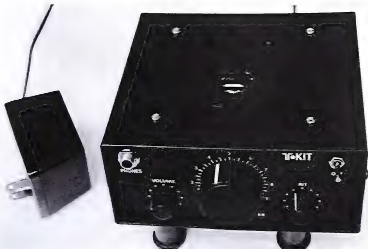
Figure 7-2 Cleverly selected and properly interfaced, "wall warts" make ideal "go anywhere" power supplies for QRP rigs in the 1 to 3 watt category. A big "wart," however, is required for 5 watt rigs.
