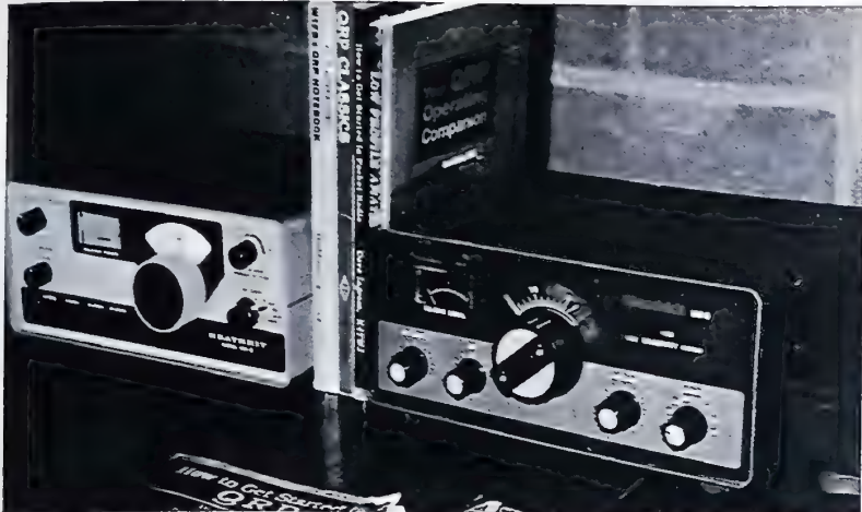
Figure 4-5 QRP and proud of it! Classic Heathkit HW-8 and HW-9 transceivers defy fading in the annals of time. Amateurs worldwide love them! Photo courtesy John Peregord, Jr., KB8UMD.
