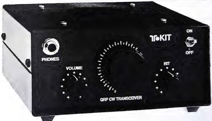
Figure 5-3 The Ten-Tec 1330 ready for action. Rig is quite small (2.7 by 6 by 6 inches, H,W,D) and delivers a clean three to four watt signal.
