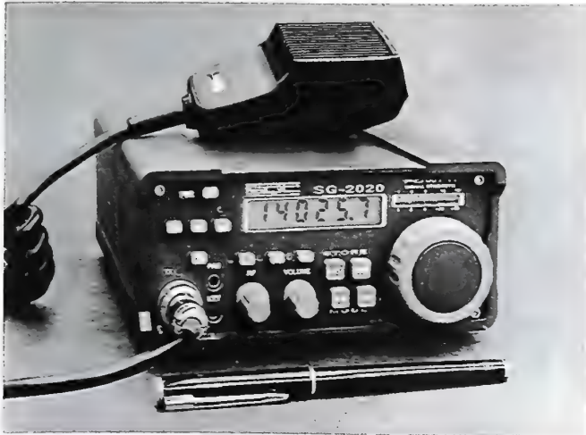
Figure 4-10 New SGC SG-2020 all band SSB/CW transceiver is remarkably small in size yet loaded with deluxe features for top-of-the-line QRP action. In many ways, it is akin to a "next generation QRP PLUS." Photo courtesy SGC, Inc.
