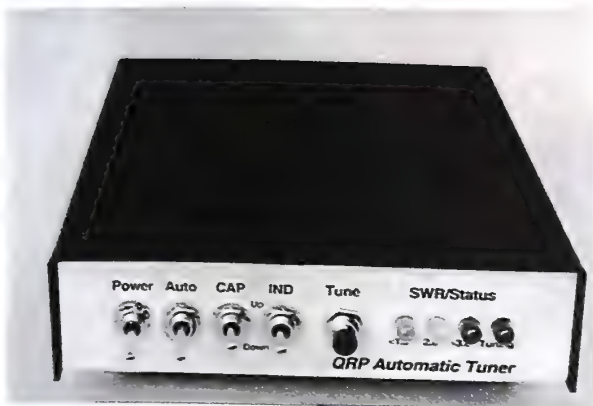
Figure 4-12 The LDG Automatic Antenna Tuner for QRP is quite small, fully microprocessor controlled, and includes LEDs for SWR metering.
