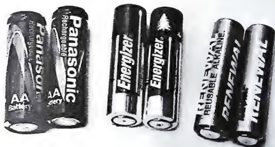
Figure 7-1 Which type cells make the best battery pack for your QRP transceiver? That depends on your operating preferences. Nickel-cadiums are low in cost for daily use, alkalines are more economical and reliable for once-a-month use, and renewable alkalines love frequent top ups for emergency preparedness. Details in text.
