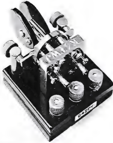
Figure 4-14 Smart looking and terrific handling "3-in-1" QRP paddle handmade by G4ZPY. Key has magnetic base for holding to a rig's case.
