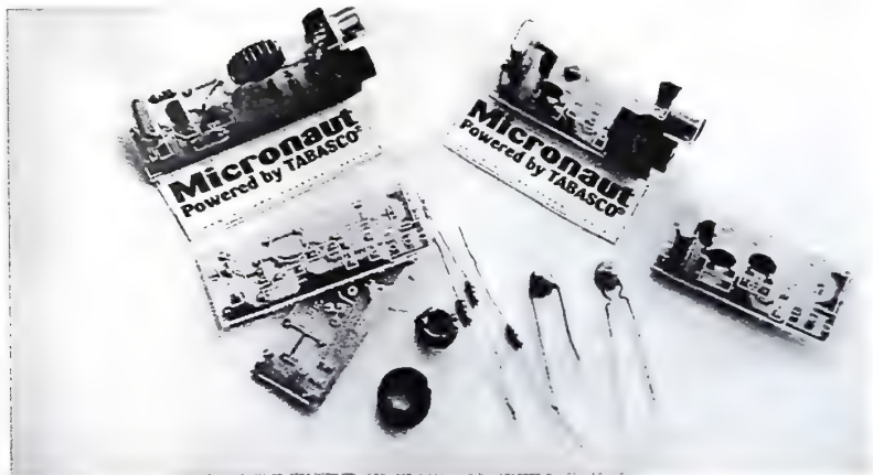
Figure 5-17 The easy-brew Micronaut transmitter kit shown in various stages of assembly. Little tyke can be powered by Tabasco sauce, grapefruits or watch batteries - a real fun project. Kits available from K4TWJ.
