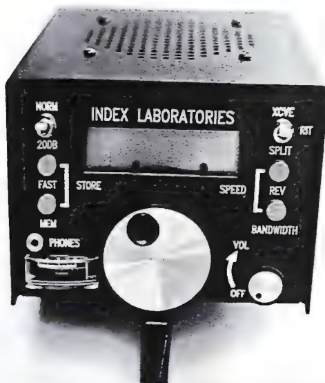
Figure 4-8 Unique-shaped QRP PLUS SSB/CW transceivers were produced by Index Labs between 1993 and 1996, and many like-new units are still in circulation today. Unit is quite deluxe, with state of the art circuitry, sharp IF filtering, narrow audio filters, programmable memories, built-in keyer, and more.
