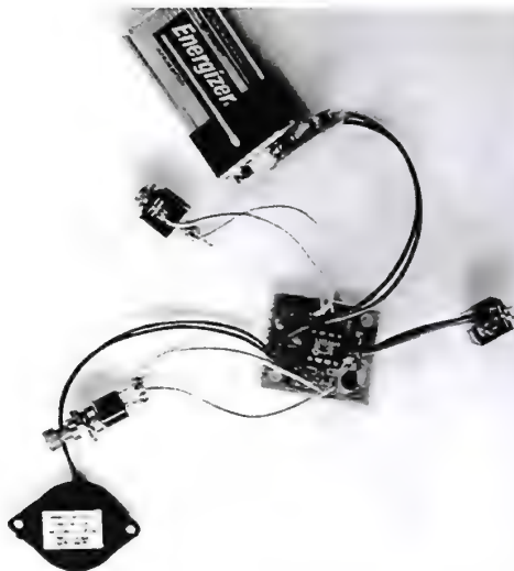
Figure 5-23 Completed Tick keyer photographed after assembly and check out. All functions like speed adjust, key/tune mode, sidetone on/off, etc., are controlled by that single pushbutton. Unit is small enough to embed in a rig, or mount in a tiny enclosure.
