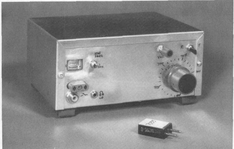
K7OWJ's compact 40 meter transceiver using the high performance direct conversion receiver described in the article. The entire unit is housed in a 3 x 5 x 7 inch box.
