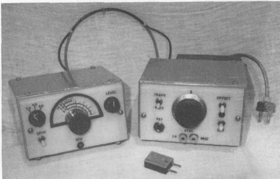
One watt transmitter and VFO by Norm Fleming, W8PJ.
