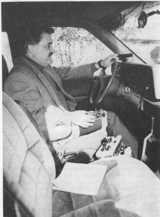
Dave Little, AF5U, with his modified paddle clamped to his leg and ready for a mobile CW QSO. His transceiver and antenna tuner can be seen between the seats of his van.
