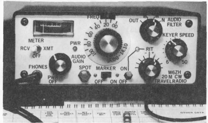
The business end of W6ZH's 20m QRP transceiver, which accompanied him on visits to VK and ZL. (Photo by W6ZH)
