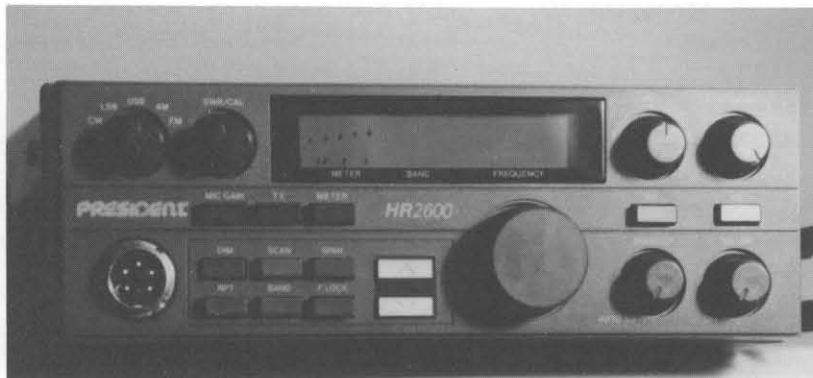
HR-2600 front panel; 20 controls and backlit LCD display.
