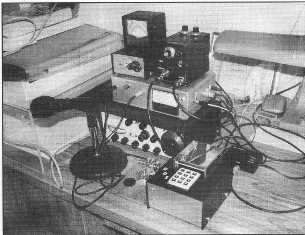
The homebrew QRP shack of Dain B. Lones, KC6WCK, includes a three-band digital readout receiver, a 5-watt DSSC transmitter with both phone and CW outputs, a cross-needle power/SWR meter, a transmatch, a direct digital synthesizer with programmable switches for each button and a T/R switch.
